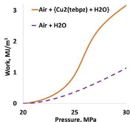
**Fig. 1. Work stored in CAES system where H<sub>2</sub>O or {Cu<sub>2</sub>(tebpz) + H<sub>2</sub>O} is used as a liquid piston**
