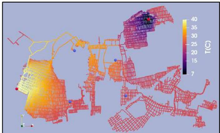
Figure 1: Mine workings beneath Durham University. Red dot represent injection points (one hot, one cold) and the blue dots abstraction points. The model is about 3 km across.
