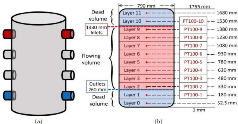
Figure 1: (a) Simplified schematic of the hot water tank, and (b) thermally stratified tank model.
