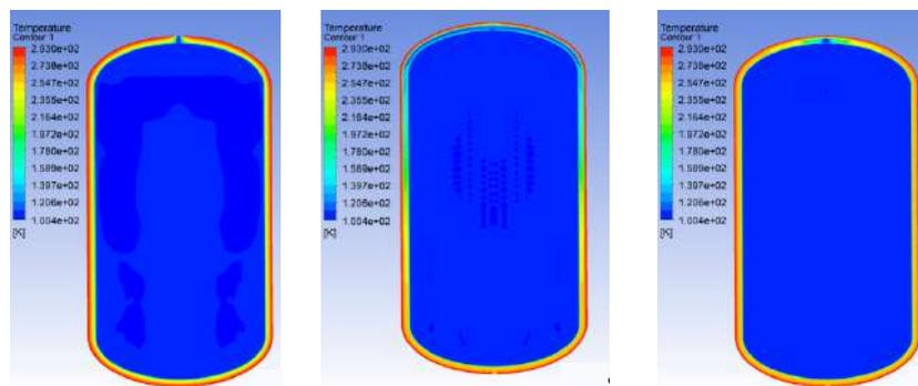
Fig.1 Temperature contours of the tank at t = 200s of structure 1, 2 and 3 from left to right
