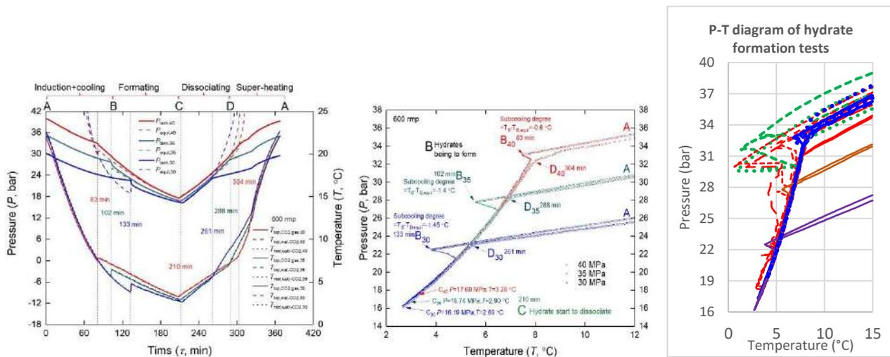
Figure 2. Tests results. Stir at 600 rpm, start pressure at 40, 35 and 30 bar (left and middle), all tests (right)
