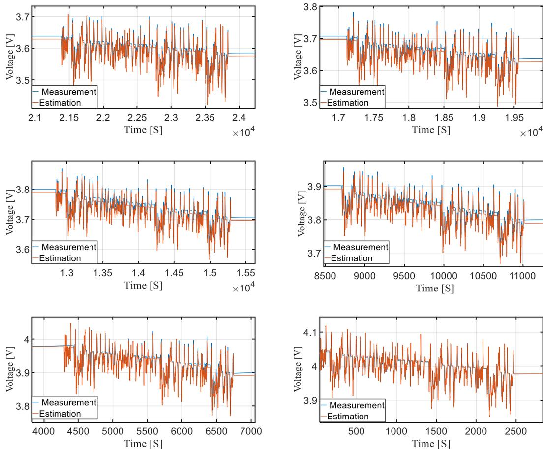
Figure 2. Comparison between estimated and measured lithium-ion battery voltage for a dynamic profile.
