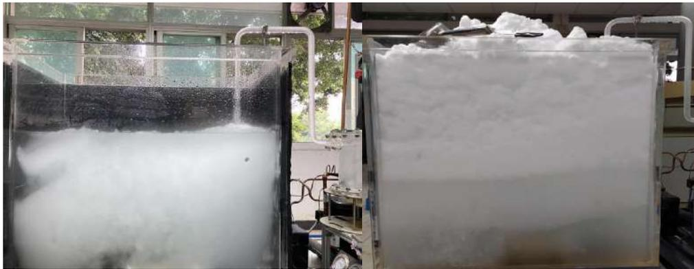
Fig. 1 Ice slurry system with supercooled water method.
