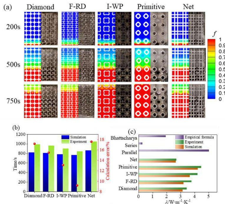
Fig. 1 (a) Liquid fraction contours of simulation and experiment results; (b) Experimental and simulation results of melting time; (c) Experimental and simulation results of the effective thermal conductivity.
