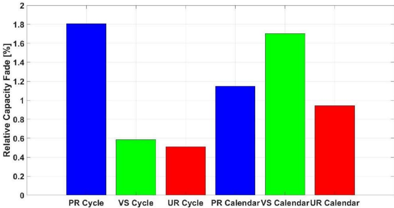
Figure 1: Cycle and Calendar Ageing applied on Primary Regulation (PR, blue bar), Voltage Support (VS, green bar) and Unbalances Reduction (UR, red bar) grid services. Time horizon simulated: 1 year.
