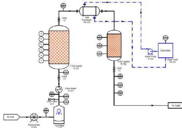
Figure 1: Schematic diagram of gas-solid packed bed TCES system
