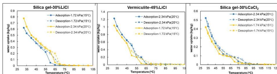
Figure 1: DSV isobars for the developed composite materials
