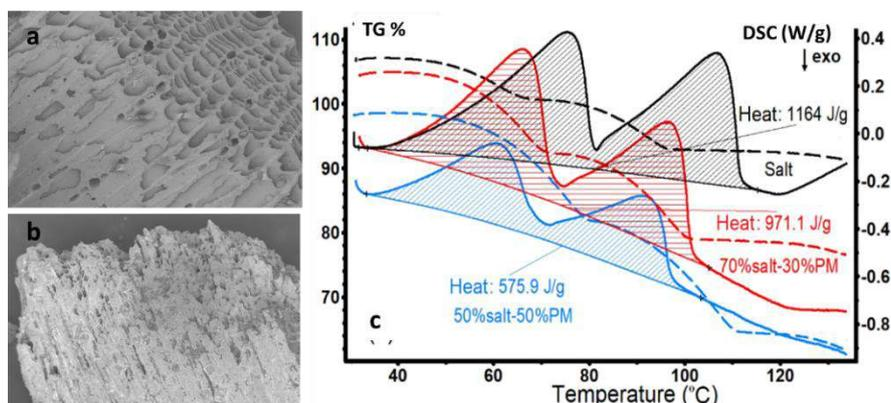
Fig 1. Microscopic images of a) porous carbon and b) impregnated salt-carbon composite as well as STA plot.
