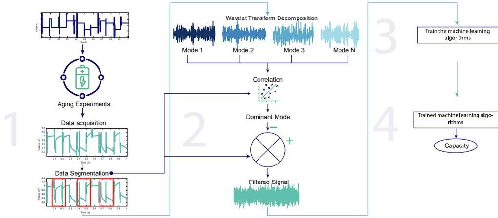
Fig. 1. The proposed framework for online capacity estimation.
