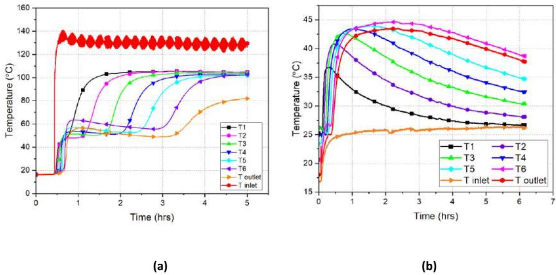
Fig 3: Experimental results for the TCES system using pure sorbent (a) Charging process (b) Discharging process
