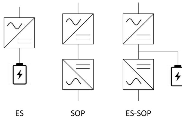
Figure 1: The topology of ES, SOP, and ES-SOP devices
