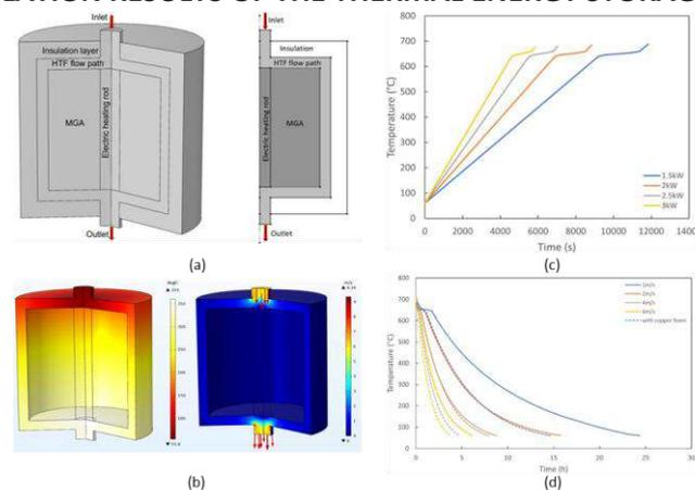
Figure 1: (a) geometry of the MGA-based thermal energy storage device; (b) temperature and velocity contours of the flow path; (c) temperature variation during charging process; (d) temperature variation during discharging process.
