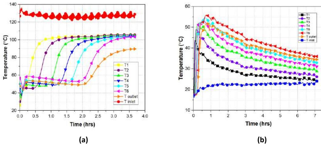
Fig 2: Experimental results for the TCES system using composite thermochemical material (a) Charging process (b) Discharging process
