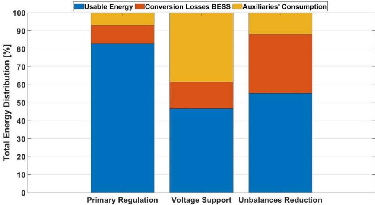
Figure 2: Total energy distribution of Primary Regulation (PR), Voltage Support (VS), Unbalances Reduction (UR) grid services. The total energy is distributed in usable energy (blue bar), conversion losses of BESS (red bar), auxiliaries' consumption (yellow bar).
