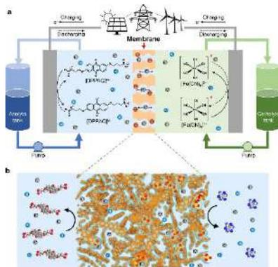
Figure 1. Aqueous organic redox flow battery for energy storage, using ion-sieving membrane with subnanometer pores that enable fast transport of charge-carrying ions while limiting the crossover of redox active species.
