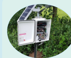
3c. Effect of different degrees of compacted soil on flooding and desiccation (using polymer tensiometers and TDR sensors)
