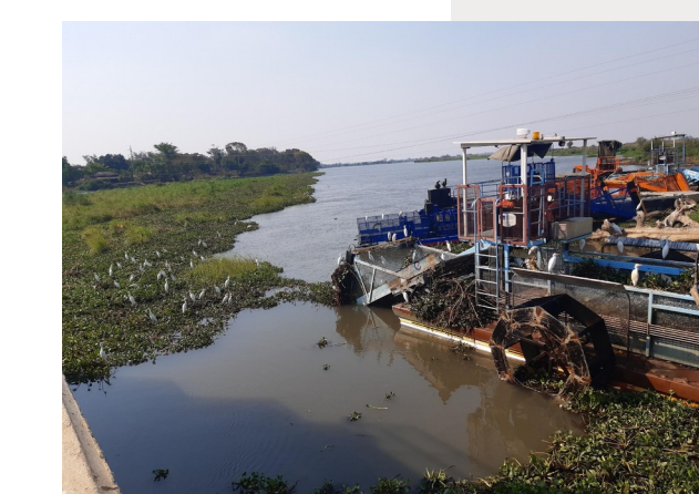
Present in most parts of the Shire River the water hyacinth (Namasipuni) is an issue for the hydropower generation. Among the fastest-growing plants, the water hyacinth impede power generation by blocking the turbines and conducting to frequent power interruptions. In a climate change context the increasing temperature may be favorable to the development of the water hyacinth (You et al. 2013)
