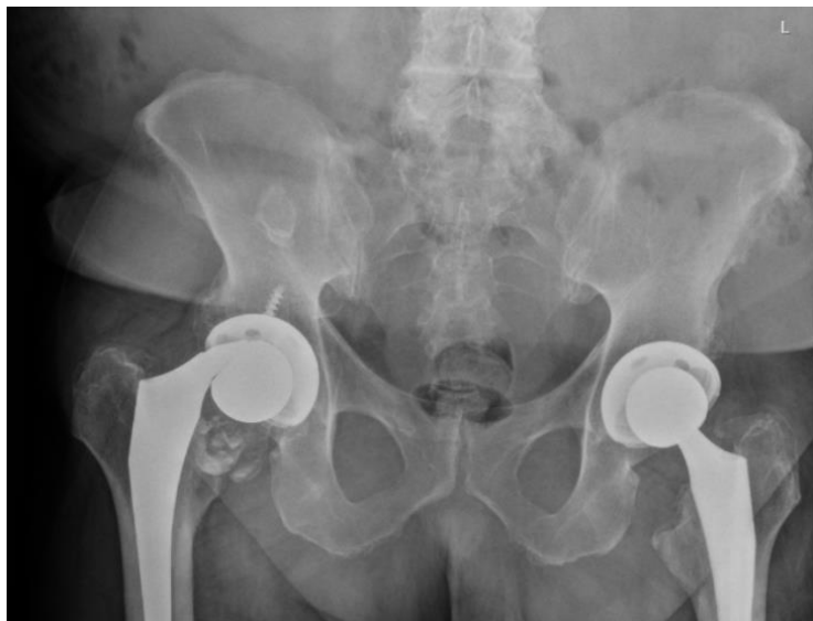
Figure 1. Radiographic Evidence of Gross Trunnion Failure. Macroscopic notching of the right femoral neck shown; image taken after admission to the emergency department.
