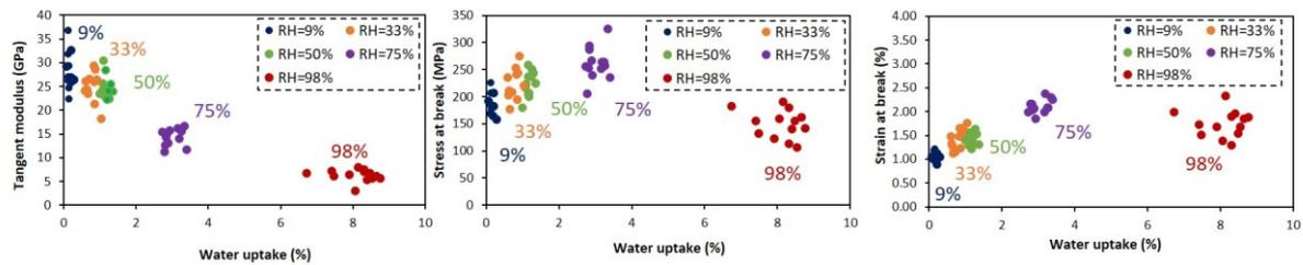
**Figure 5.** Evolution of the performances of hemp/epoxy composites as a function of water sorption.
