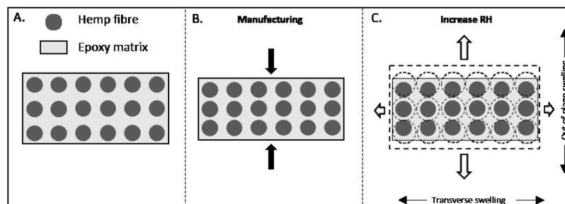
**Figure 3.** Schematic representation of dimensional variation of hemp/epoxy composite between initial state (A), after manufacturing (B) and after increasing the relative humidity.
