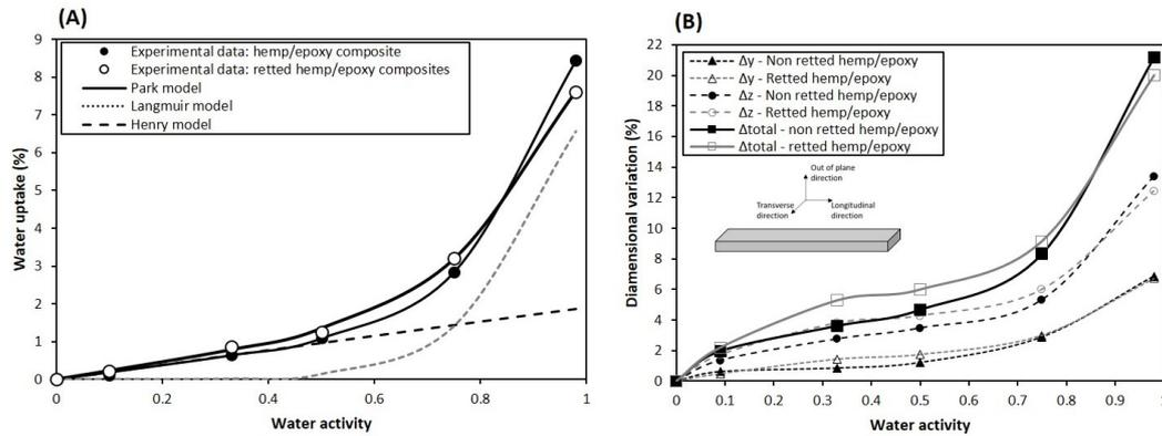
**Figure 1.** (A) Water vapor isotherm at 25° of non-retted and retted hemp/epoxy composites. Park model is used to fit experimental data and deconvoluted into Langmuir, Henry and clustering components. (B) Transverse swelling ( $\Delta y$ ), out of plane swelling ( $\Delta z$ ) and total swelling of non-retted and retted hemp/epoxy biocomposites over a range of water activity 0.09 and 0.98.
