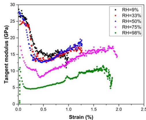
**Figure 4.** Evolution of tangent modulus with the longitudinal strain of hemp/epoxy UD composites saturated at different relative humidity: 9%, 33%, 50%, 75%, 98%.
