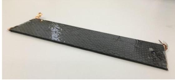
**Figure.1** As prepared graphene coated carbon fabric composite
