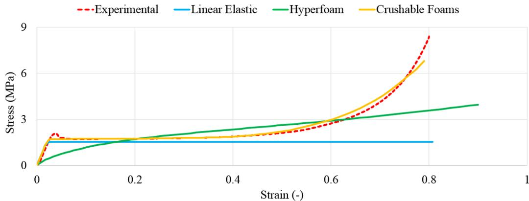
**Figure 7.** Compressive stress-strain comparison between experiment and FEA.
