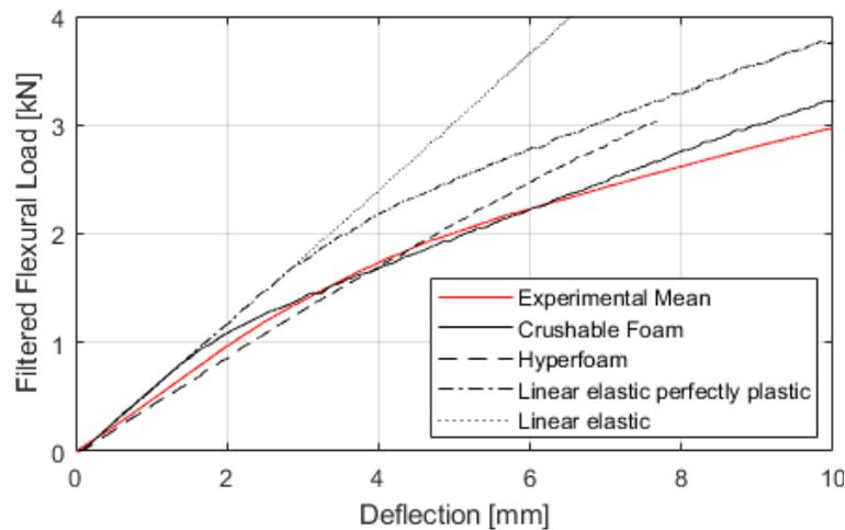
**Figure 8.** Sandwich beam load-deflection comparison between experiment and FEA.
