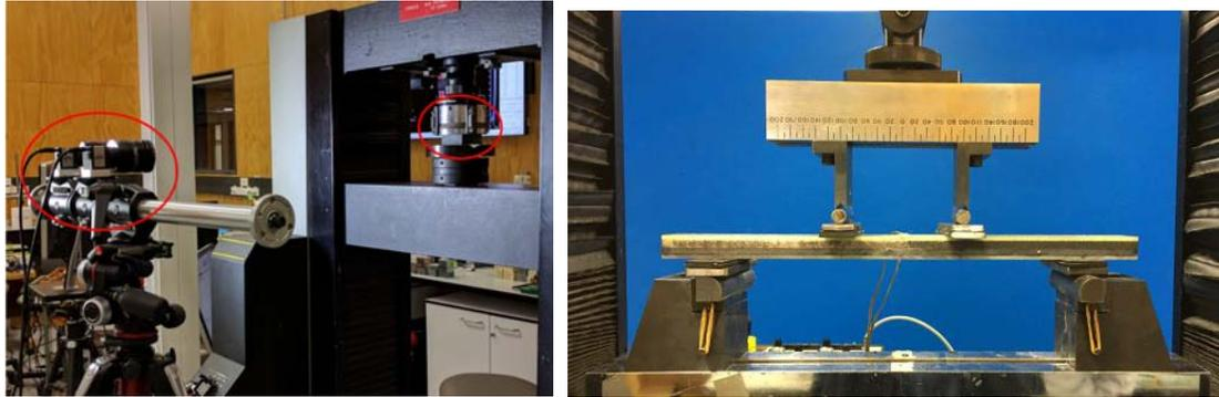
**Figure 1.** Compression testing setup with DIC cameras. **Figure 2.** Four point loaded beam test setup.
