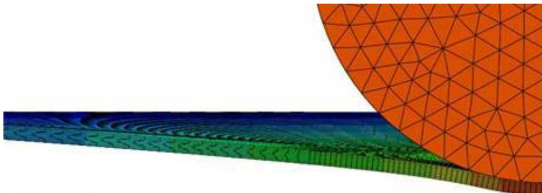
**Figure 10.** Local deformation of sandwich panel during hard-body impact.
