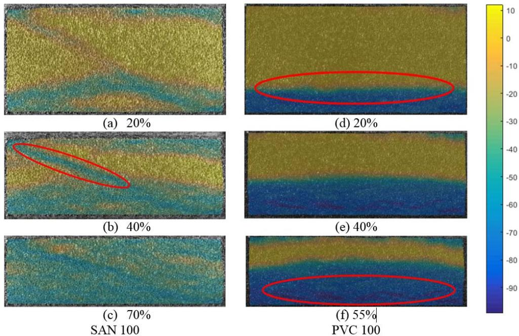
**Figure 6.** DIC strain results for SAN and PVC foam during through thickness compression tests (%).
