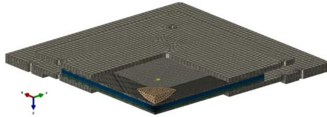
**Figure 5.** Quarter panel impact model with fixtures.
