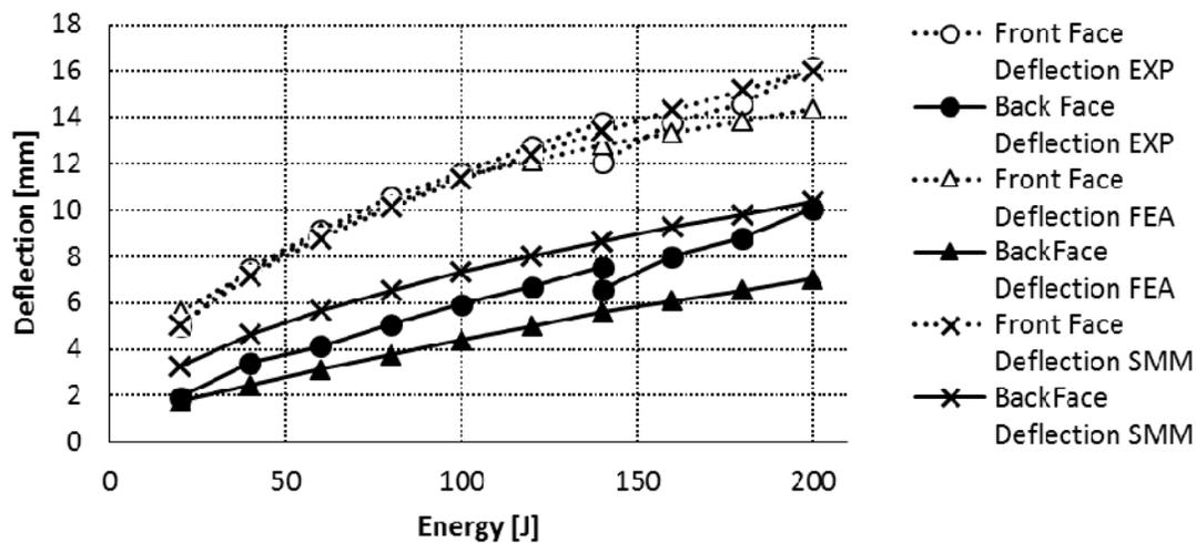
**Figure 9.** Front and back-face transverse deformations of sandwich panel during hard-body impact including experimental, FEA and analytical solutions.
