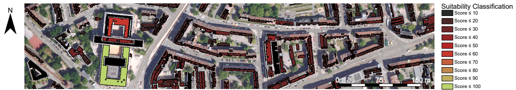
Fig. 1: Homogeneous roof areas of a subset of the study area. Background map from Bayerische Vermessungsverwaltung (2026). Note the high suitability of the green-shaded, flat, and mostly homogeneous rooftop.
