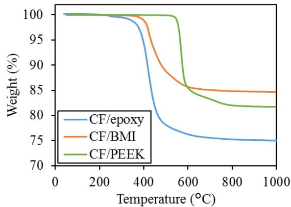
**Figure 4.** Thermogravimetric analysis results for CF/epoxy [9], CF/BMI and CF/PEEK in argon gas flow. The heating rate was 20°C/min.
