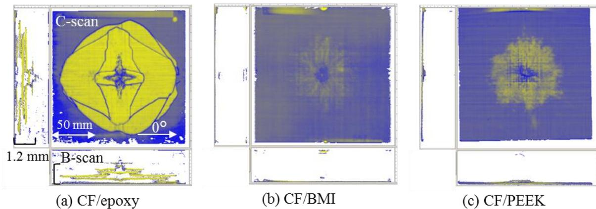
**Figure 3.** Non-destructive inspection results using ultrasonic technique.
