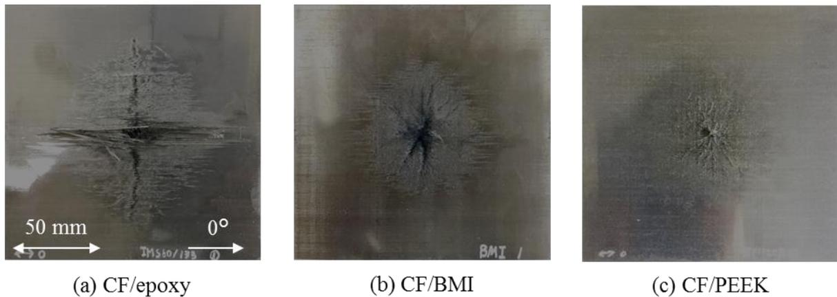
**Figure 2.** Arc attachment surface.
