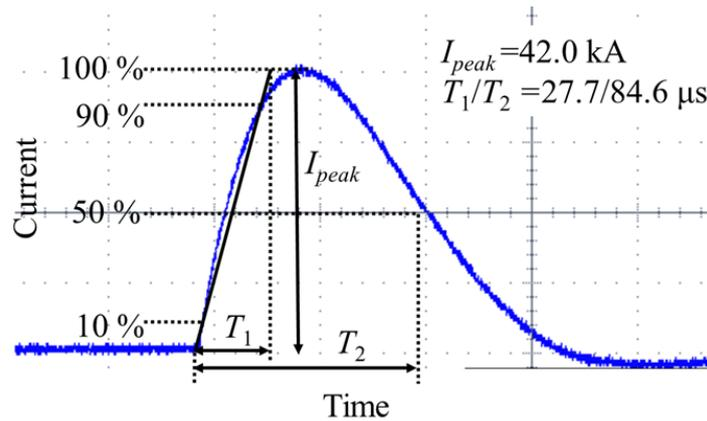
**Figure 1.** Typical lightning waveform.
