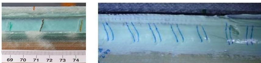
**Figure 6.** Damage initiation. Left: Vertical cracks in the beam adhesive bond line. Right: Vertical cracks in a WTRB spar to shear web bond line
