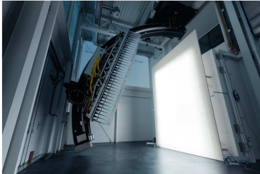
Fig. 2: The artificial sun, comprising the illuminator mounted on a rotating 90 degrees arc-rail, illuminates a screen in front of the test chamber during testing (image courtesy Girts Apskalns).
