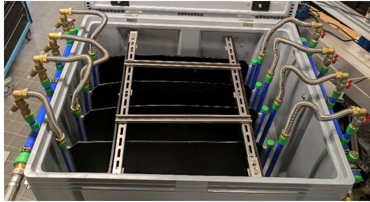
Fig. 2: Photo of the experimental GSHX box in the laboratory environment.
