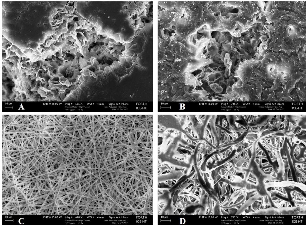
Figure 1- SEM images of scaffolds: a) PCL solvent cast film (PCL SC), b) PCL-CNTs solvent cast film (PCL-CNTs SC), c) PCL electrospun film (PCL ES) and d) PCL-CNTs electrospun film (PCL-CNTs ES).
