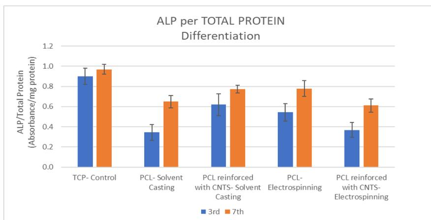
**Figure 3- Cell Differentiation: Measurement of Total Protein Levels in 3 and 7 days of cell culture on PCL - Solvent Casting, PCL reinforced with CNTs - Solvent Casting, PCL - Electrospinning and PCL reinforced with CNTs – Electrospinning.**
