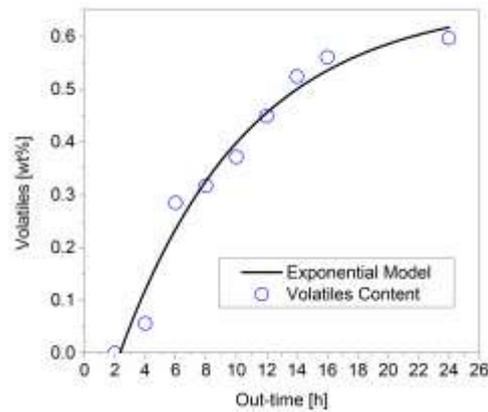
Figure 2 Volatile content modelled as a function of out-time using linear and exponential relations
