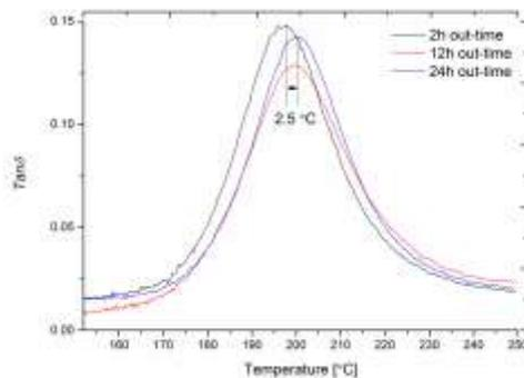
Figure 5 DMA tests of laminates manufactured from tapes exposed to out-time from 2h, 12h and 24h out-time, showing negligible change in  $T_g$  loss modulus peaks
