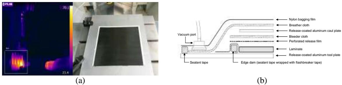
Figure 1 Composite manufacturing using an in-house AFP rig (a) Manufacturing set-up and a sample laminate on a Bridgeport® milling table (b) Bagging sequence used to cure the laminate after layup
