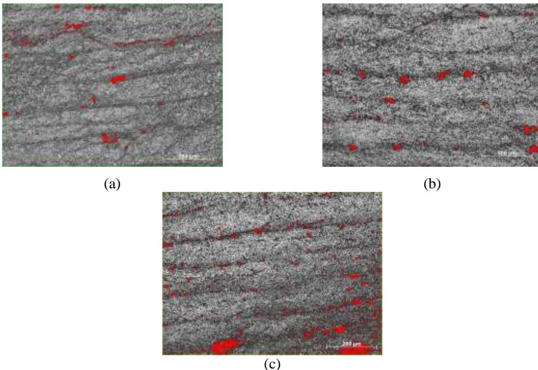
Figure 3 Micrograph of the cross-section of a  $[0/\pm 45/90]_s$  laminate manufactured from prepregs subjected to (a) 2h out-time with voids highlighted in red which is approximately 1.3% of the  $0.576 \text{ mm}^2$  measured area (b) 12h out-time with voids highlighted in red which is approximately 1.5% of the  $0.576 \text{ mm}^2$  measured area (c) 24h out-time with voids highlighted in red which is approximately 2.5% of  $0.571 \text{ mm}^2$  measured area
