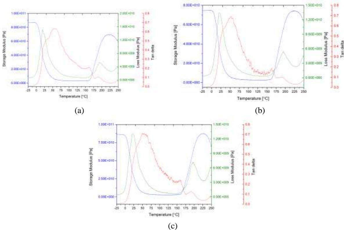
Figure 4 DMA test results of CYCOM 5320-1 tapes exposed to (a) 2h out-time (b) 12h out-time (c) 24h out-time
