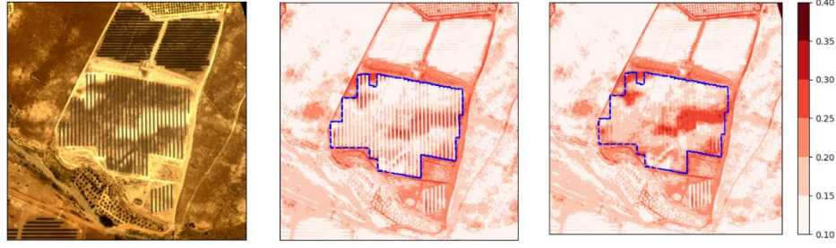
Figure 1: Raw WorldView image of a PV plant near Tabernas, Spain (left), ground albedo map (center) and albedo map in which PV modules and shades were removed (right). The solar field's footprint is indicated by a blue dashed polygon.
