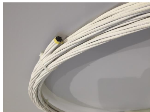
Fig. 7 Photo of 'CABKOMA™ STRAND ROD', a CFRTP rod using thermoplastic epoxy resin manufactured by Komatsu Seiren Co. Ltd.
