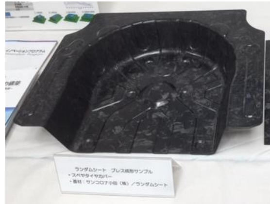
Fig. 8 Photo of a spare tire cover molded by using 'Flexcarbon TM ', a thin-layered random stampable sheet manufactured by SUNCORONA ODA Co. Ltd.
