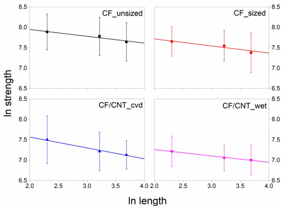
**Figure 2.** Experimentally derived relationships of the fibre strength with respect to the fibre length.
