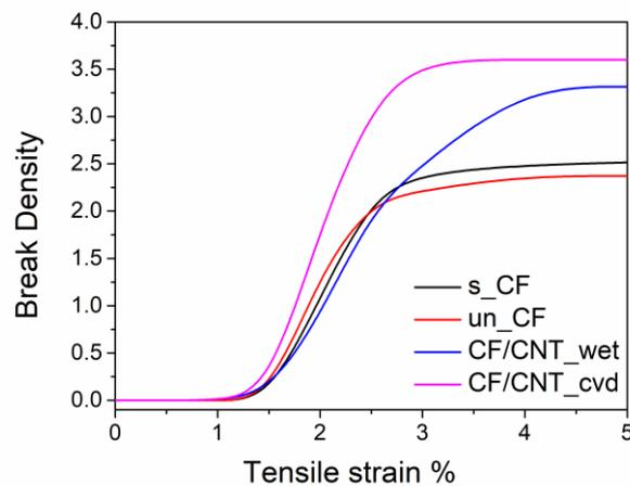
**Figure 3.** Characteristic Break density vs tensile strain plots for the reference and hierarchical CFs as measured by SFFT.
