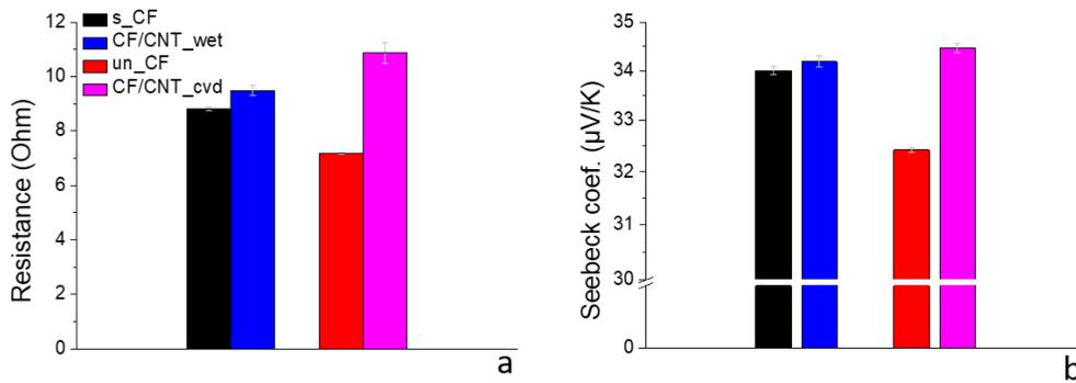
**Figure 4.** a) Electrical resistance and b) Seebeck coefficient of the reference and the hierarchical CFs.
