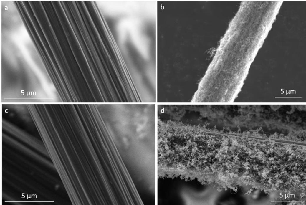
**Figure 1.** SEM micrographs of the reference and the hierarchical CFs, a) s\_CF, b) CF/CNT\_wet, c) un\_CF and d) CF/CNT\_cvd.
