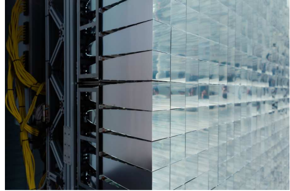
Fig. 1: Left: PCB with 26 LEDs in its centre, emitting in the visible (cold and warm white) and near infrared ranges. Right: Array of C-CPCs with attached PCBs forming the illuminator of the Artificial Sun (image courtesy Girts Apskalns).
