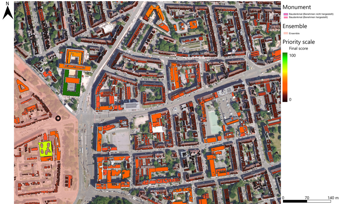
Fig. 7: Final solar cadastre showing the priority score for suitable roof segments and overlaid heritage-protected areas. Background: Bayerische Vermessungsverwaltung – https://www.geodaten.bayern.de (data modified), CC BY 4.0.
