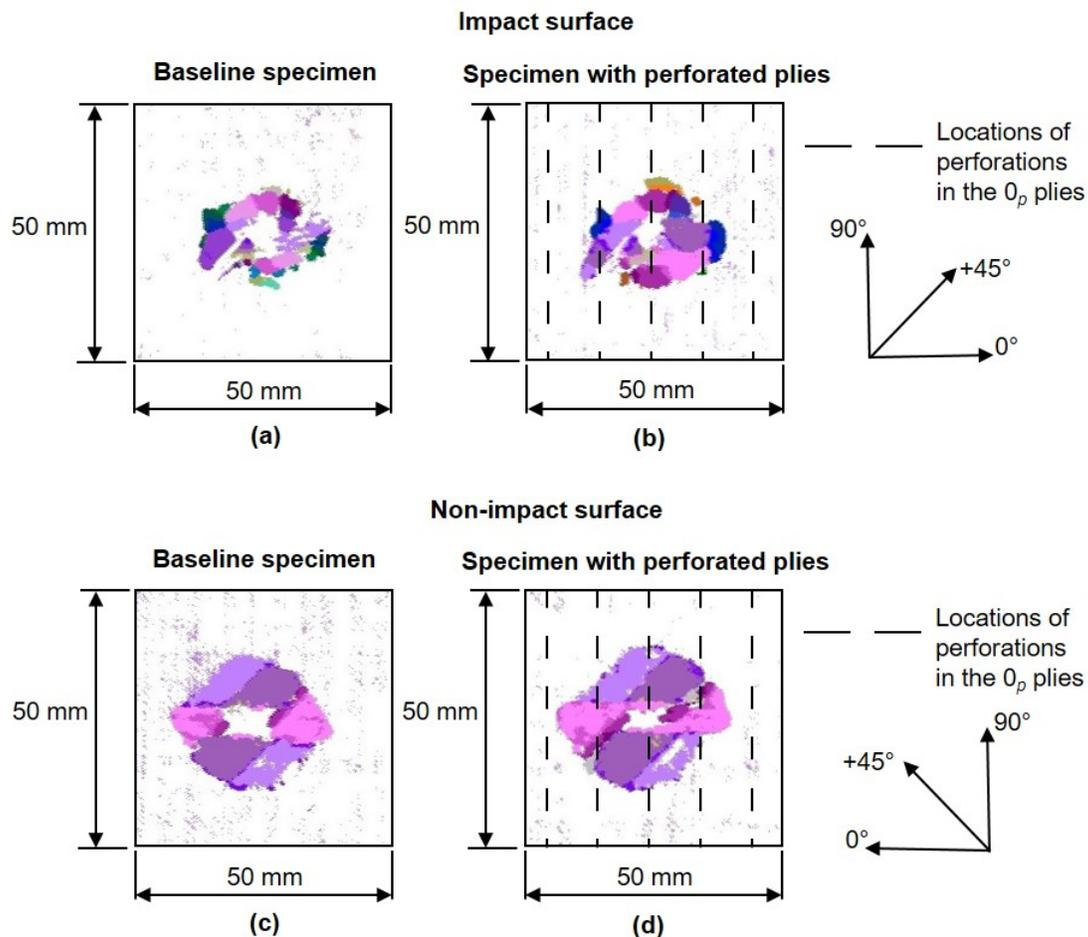
**Figure 3.** C-scan images of the impact surface of a baseline specimen (a) and a specimen containing ply perforations (b) and of the non-impact face of a baseline specimen (c) and a specimen containing ply perforations (d).
