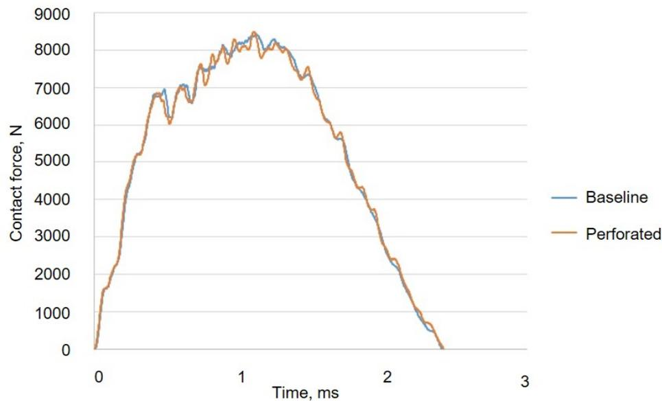
**Figure 2.** Impact force as a function of time during the impact event for a representative baseline specimen and a representative specimen containing ply perforations.
