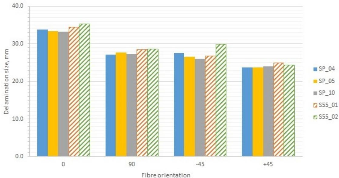
**Figure 4.** Maximum size of delamination measured along the 0, 90, -45 and +45 fibre orientation in C-scan images of the non-impact face of all the specimen tested. ‘SP\_’ represents specimens without perforations, ‘S55\_’ represents specimens containing 5-mm-long perforations/5-mm continuous fibres.
