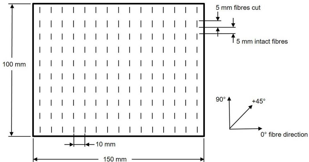
**Figure 1.** Schematic representation of the plan view of a perforated 0<sub>p</sub> ply.
