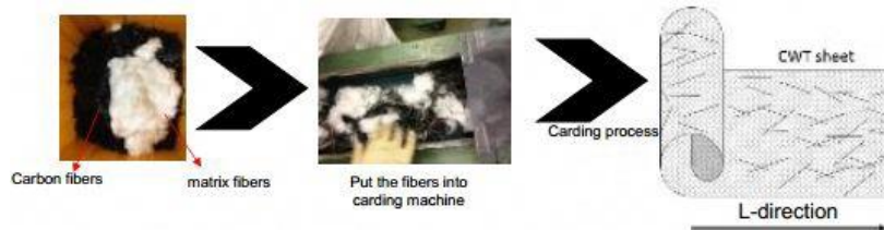
Figure 4. The carding process for CWT sheets [8]
