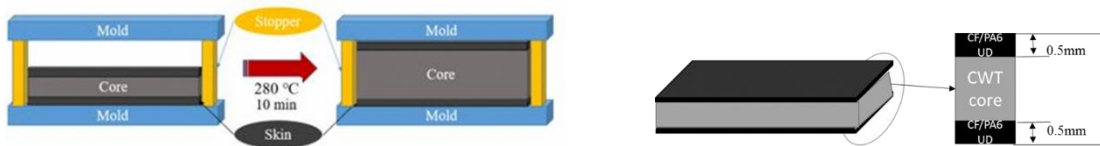
Figure 3. Manufacturing process for springback sandwich structures
