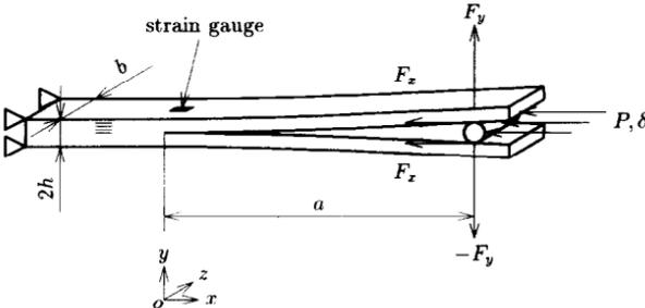
Figure 2. A wedge insert fracture specimen from [9].
