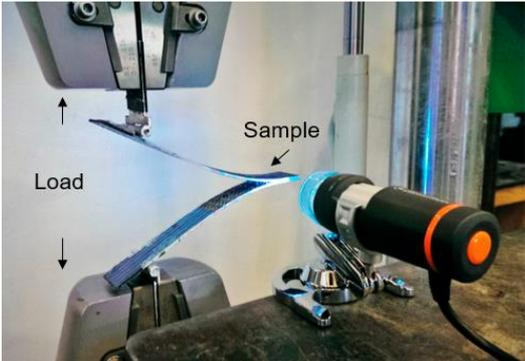
Figure 3. DCB testing set up using INSTRON 5966
