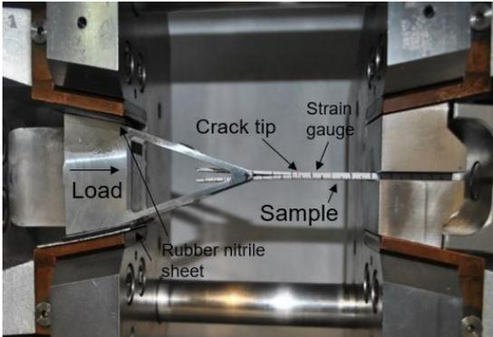
Figure 4. Wedge insert fracture testing setup using Gleeble 3800-GTC.
