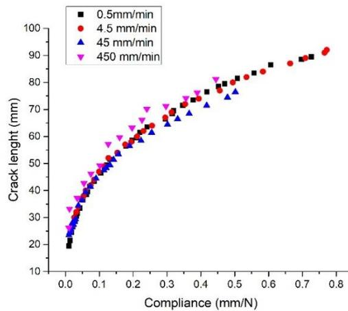
**Figure 5** Relation between compliance and crack length
