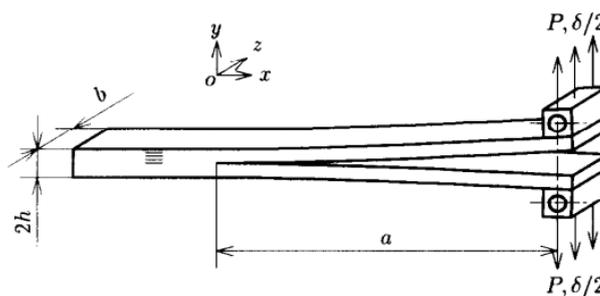
**Figure 1.** A double cantilever beam specimen from [9].
