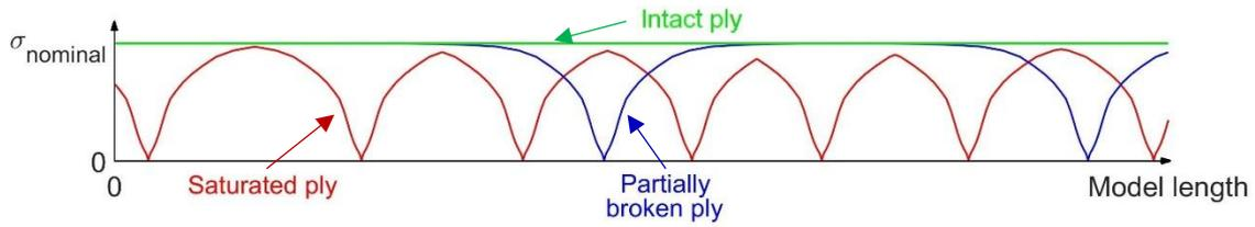
**Figure 2** – Stress state of the carbon ply in its intact, partially broken and saturated state.
