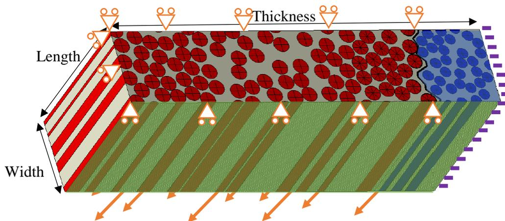
**Figure 1** – FE model design and applied boundary conditions. The blue surface is the cracked surface and the green face is subjected to periodical conditions to the opposite side. Thickness symmetry is represented by the purple lines.
