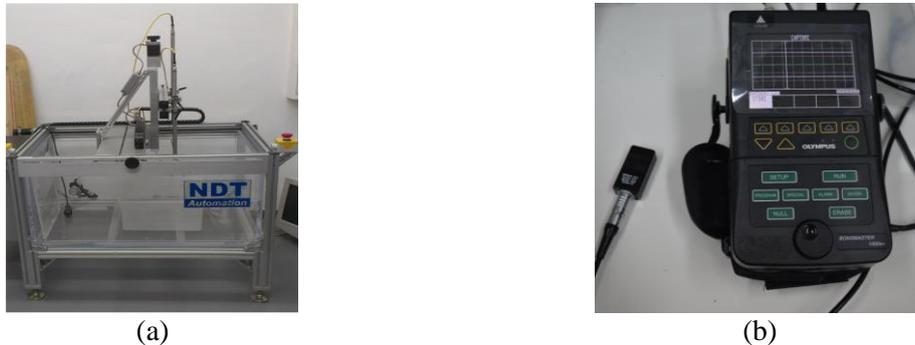
**Figure 7.** Non destructive testing apparatus. (a) Ultracac II by Mistras Group. (b) Olympus Bondmaster.
