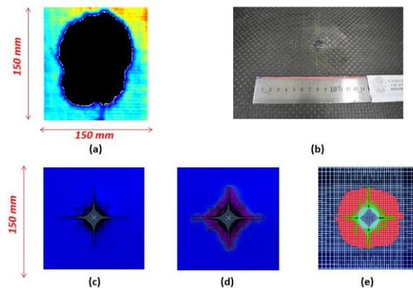
**Figure 10.** Correlation of damage footprint of impacted plate at 96 m/s (case 3). (a) Post-Impact C-scan. (b) Front side of the impacted plate. (c) Fiber damage (Deleted Elements). (d) Delamination (Cohesive). (e) Matrix damage.
