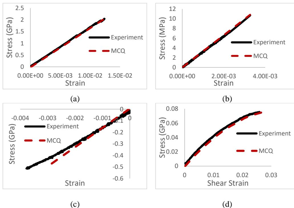
**Figure 2.** Material modeling verification through static tests on UD specimens. (a) Longitudinal Tension. (b) Transverse Tension. (c) Longitudinal Compression. (d) Shear Tension.
