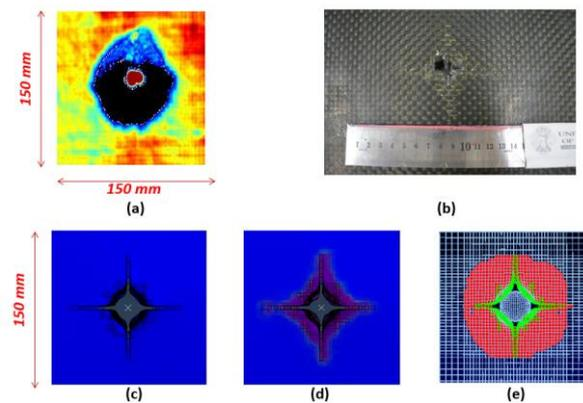
**Figure 9.** Correlation of damage footprint of impacted plate at 80 m/s (case 2). (a) Post-Impact C-scan. (b) Front side of the impacted plate. (c) Fiber damage (Deleted Elements). (d) Delamination (Cohesive). (e) Matrix damage.
