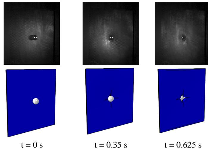
**Figure 11.** Screenshots of impact test and numerical impact simulation on the woven carbon/epoxy plate 300x300x5mm with 30mm steel ball at 96 m/s.
