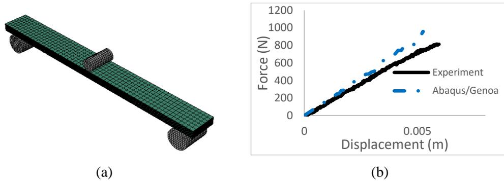
**Figure 3.** Multi-scale progressive failure simulation of three-point bending on woven specimen. (a) 3-D continuum explicit FEA model. (b) Force-Displacement curve.
