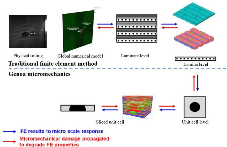
**Figure 1.** Graphical presentation of the multi-scale progressive failure analysis.
