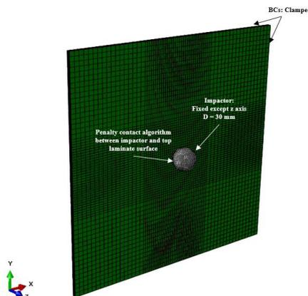
**Figure 4.** 3D continuum FE model used for the numerical validation of impact event.
