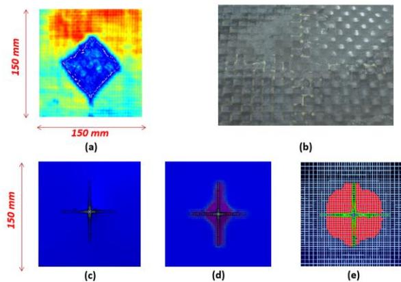
**Figure 8.** Correlation of damage footprint of impacted plate at 56 m/s (case 1). (a) Post-Impact C-scan. (b) Front side of the impacted plate. (c) Fiber damage (Deleted Elements). (d) Delamination (Cohesive). (e) Matrix damage.
