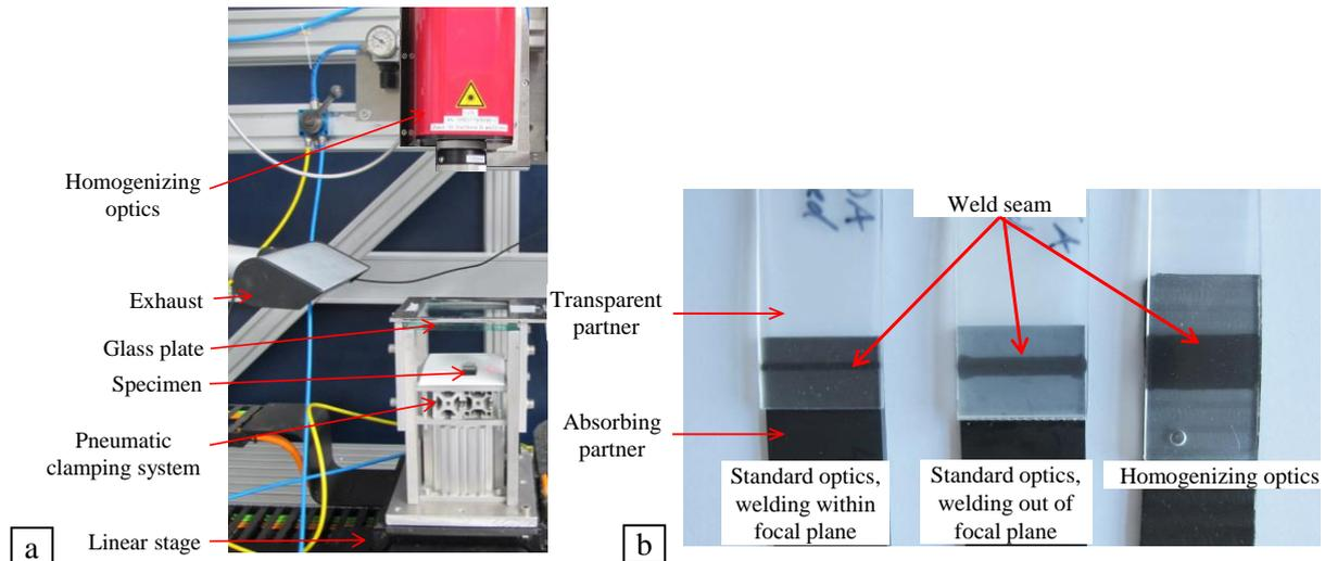
**Figure 2.** (a) Experimental setup with homogenizer optics and (b) weld seam geometry for different optics and focal plane settings.
