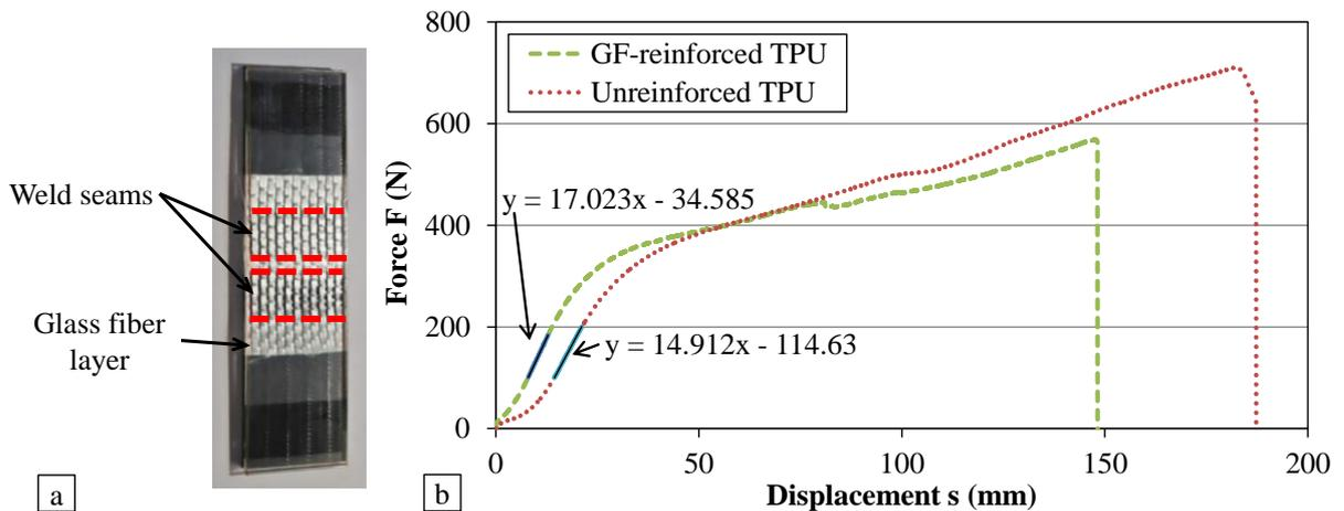
**Figure 10.** (a) Glass fiber reinforced specimen and (b) force-displacement curve for tensile testing of reinforced and unreinforced specimens
