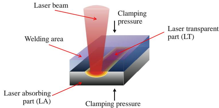
**Figure 1.** Laser transmission welding principle.
