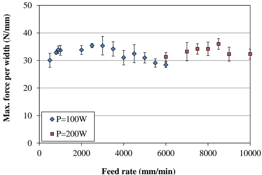
**Figure 6.** Maximum force obtained for varying laser power and feed rate at a constant spot size of  $A = 10 \times 10 \text{ mm}^2$  and clamping pressure of  $p = 3 \text{ bar}$ .
