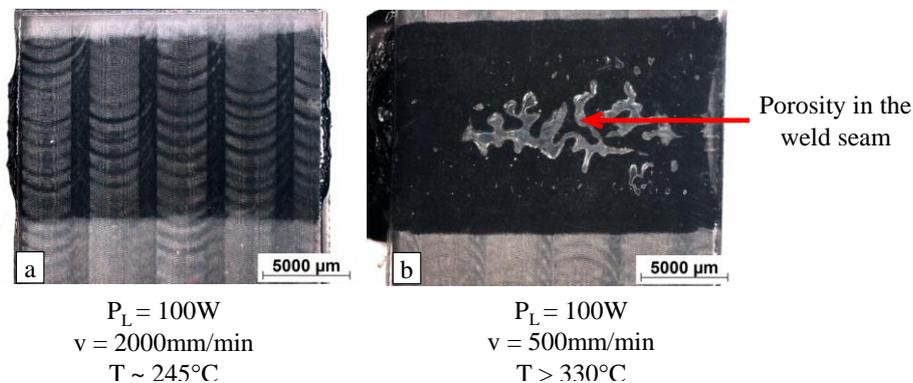
**Figure 7.** Exemplary weld seam appearance for an ideal welding parameter set (a) and a parameter set leading to overheating (b).
