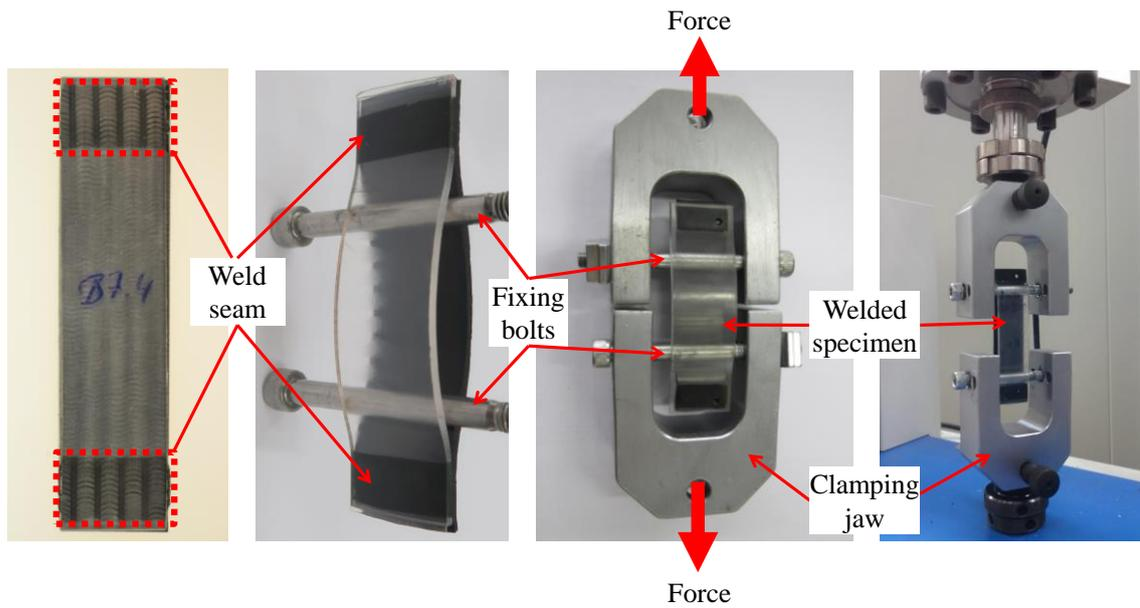
**Figure 5.** Tensile testing specimen and setup.
