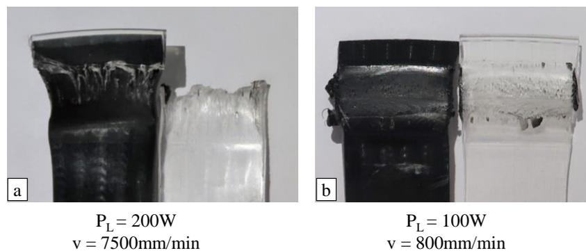
**Figure 8.** Exemplary fracture appearance for an ideal welding parameter set (a) and a parameter set leading to overheating (b).
