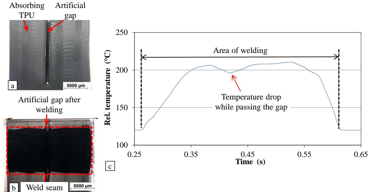
**Figure 9.** Defect simulation; (a) artificial gap before welding, (b) gap after welding, (c) temperature profile during welding, passing an artificial gap.
