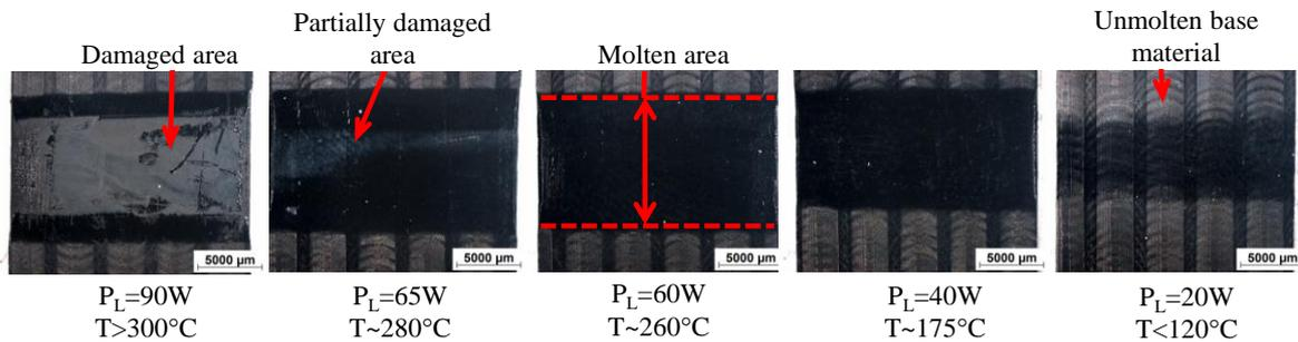
**Figure 4.** Bead-on-plate weld results with corresponding laser power and temperature measurements.
