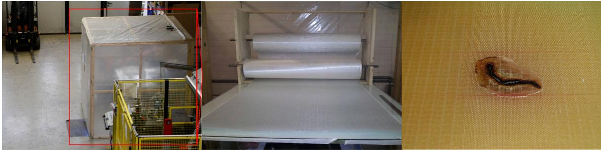
Figure 7: **Left and middle:** carbon-fiber-free environment used for GFRP preforming.
