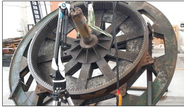
Figure 1. Case study: internal large-scale spur gear
