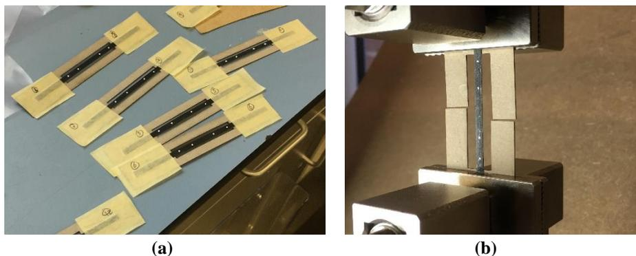
**Figure 5:** (a) Preparation of tensile samples and (b) samples loaded between grips.
