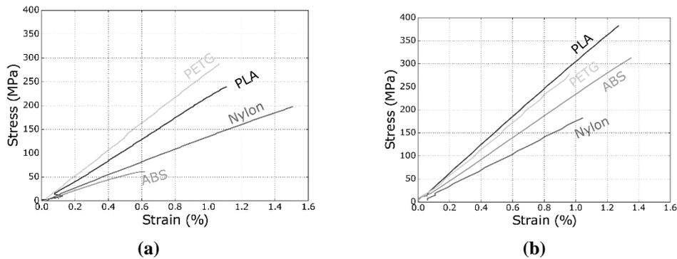
**Figure 6:** Stress-strain curves of ADFRTPs at (a) low processing temperature and (b) high processing temperature.
