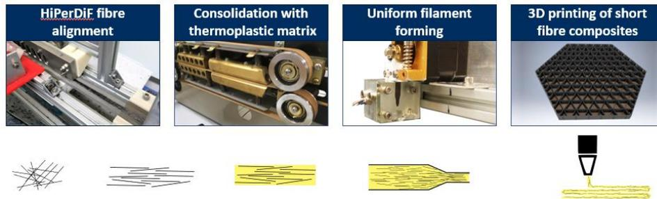
**Figure 2:** Four main processing steps from dry fibres to 3D printing filament.
