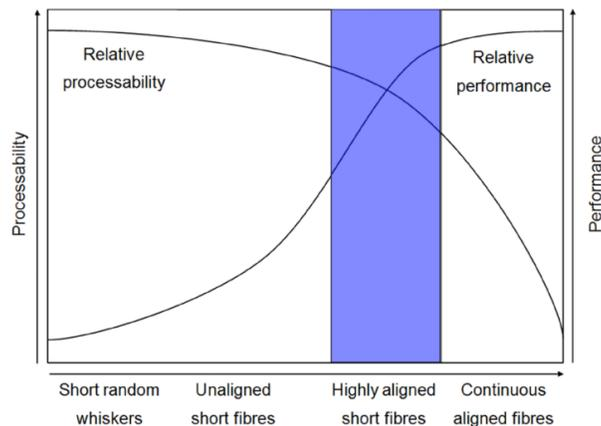
**Figure 1:** Balance between process ability and performance for different fibre architectures [8].
