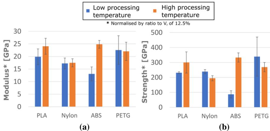
**Figure 7:** Tensile test results of ADFRTP processed at different temperature, normalized by ratio to a  $V_f$  of 12.5%.
