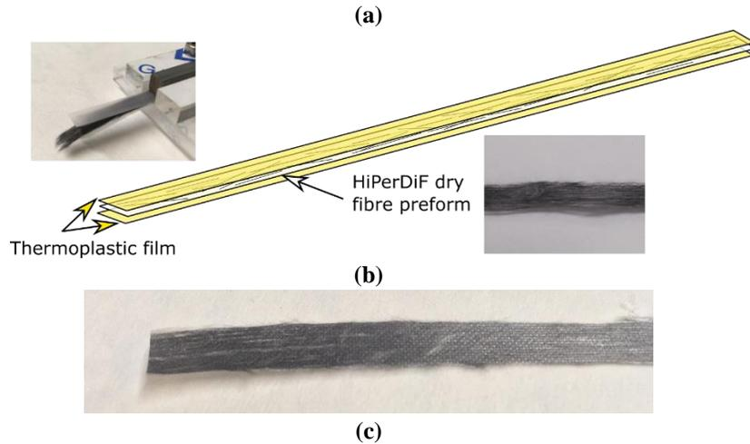
**Figure 4:** (a) Consolidation module showing (b) the fibre and matrix preforms before processing and (c) after processing.
