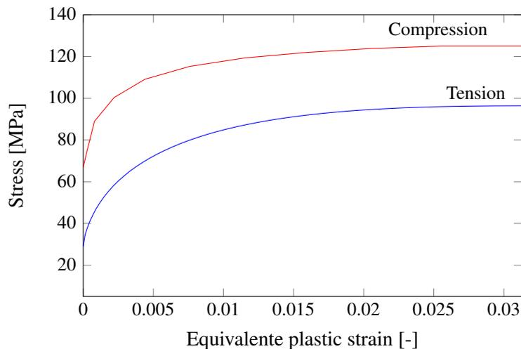
**Figure 4.** Input hardening curves for plasticity model.
