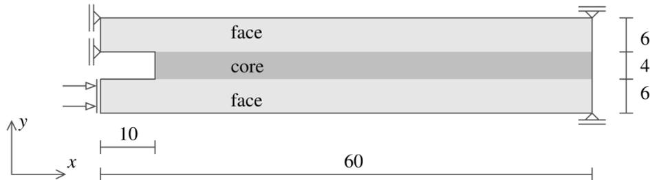
**Figure 3.** Rail shear test (dimensions in mm) [4].
