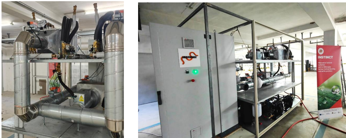
Fig. 2: Experimental prototype of the adsorption-based atmospheric water harvesting system
