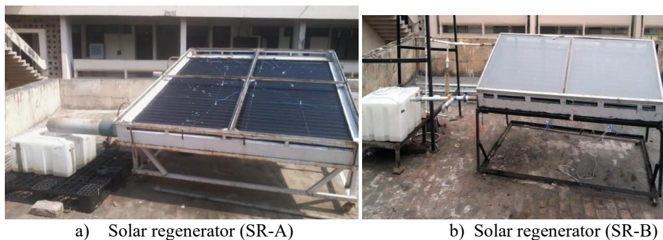
Figure 1. The experimental solar thermal brine regenerators
