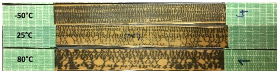
**Figure 4.** Typical specimens showing the damage pattern of thin continuous glass/carbon hybrid specimens after testing at various temperatures
