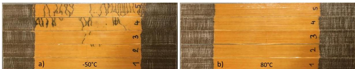
**Figure 7.** Damage mode of the thick, discontinuous specimens at a) -50°C and b) 80°C (Behaviour at 25°C was similar to that at 80°C)
