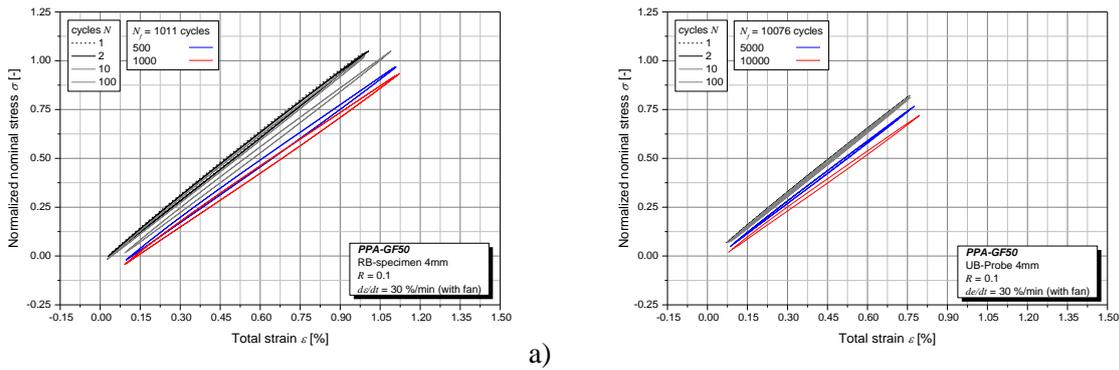
Figure 6. test results for  $R = 0.1$  at: a)  $\Delta\varepsilon_a = 0.5\%$ ; b)  $\Delta\varepsilon_a = 0.35\%$
