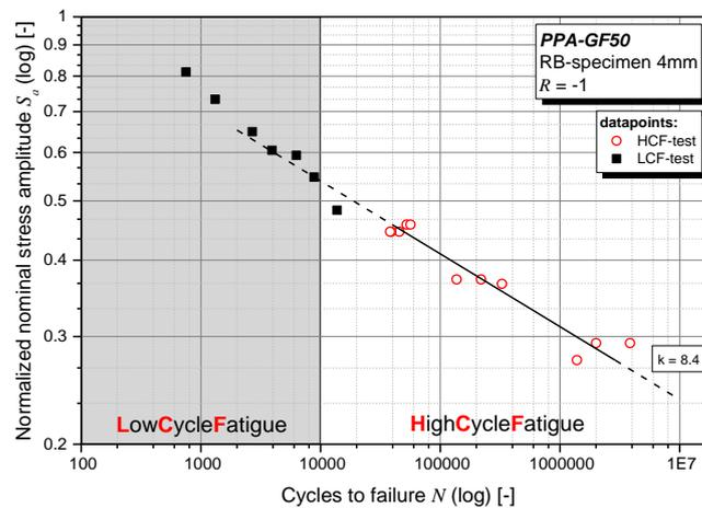
**Figure 8.** compared test results for  $R = -1$
