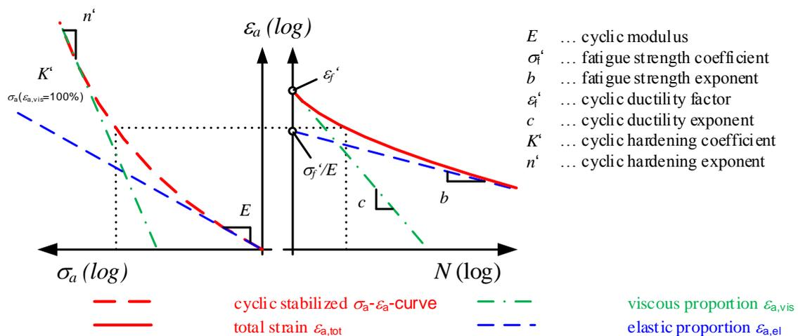
Figure 2. cyclic stabilized  $\sigma/\varepsilon$ -curve and  $\varepsilon/N$ -curves
