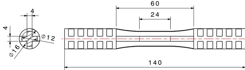
Figure 4. unnotched rotary bending specimen according to [9]
