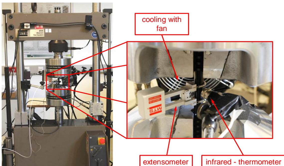
Figure 3. test setup for strain controlled tests
