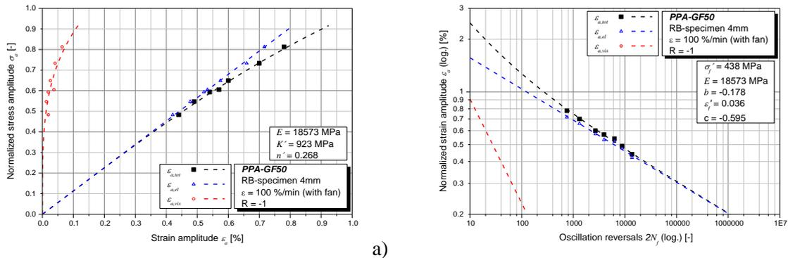
Figure 7. test results for  $R = -1$ : a) cyclic stabilized  $\sigma$ - $\varepsilon$ -curve; b)  $\varepsilon/N$ -curves
