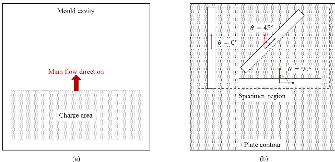
**Figure 1.** Specimen manufacturing: (a) initial material placement before compression moulding, and (b) moulded plate after compression moulding. Red arrows indicate, in both figures, the main flow direction.
