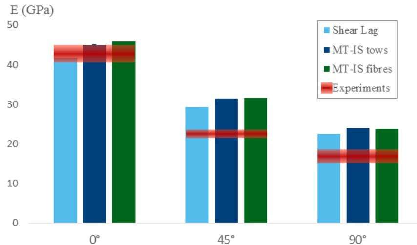
**Figure 3.** Results of model predictions compared to experimental results
