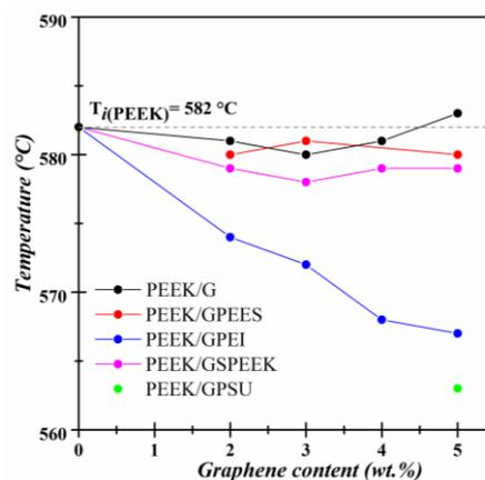
**Figure 1.** Variation of the initial degradation temperature,  $T_i$ , obtained at a 5% weight loss, with graphene loading under nitrogen atmosphere. Values for pure PEEK are indicated by a dash line.
