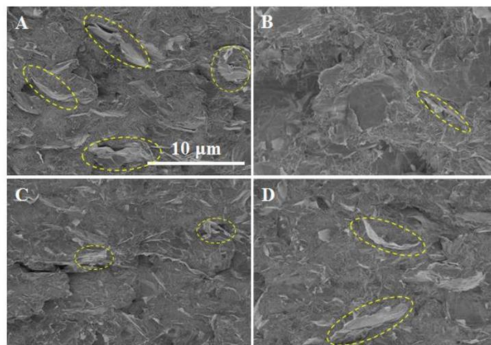
**Figure 2.** SEM micrographs of cryo-fractured films of PEEK nanocomposites with a 5 wt.% of G: PEEK/G (A), PEEK/GPEI(B), PEEK/GSPEEK (C) and PEEK/GPEES(D). All the images were collected with the same magnification. Yellow ellipses are enclosing some graphene aggregates.
