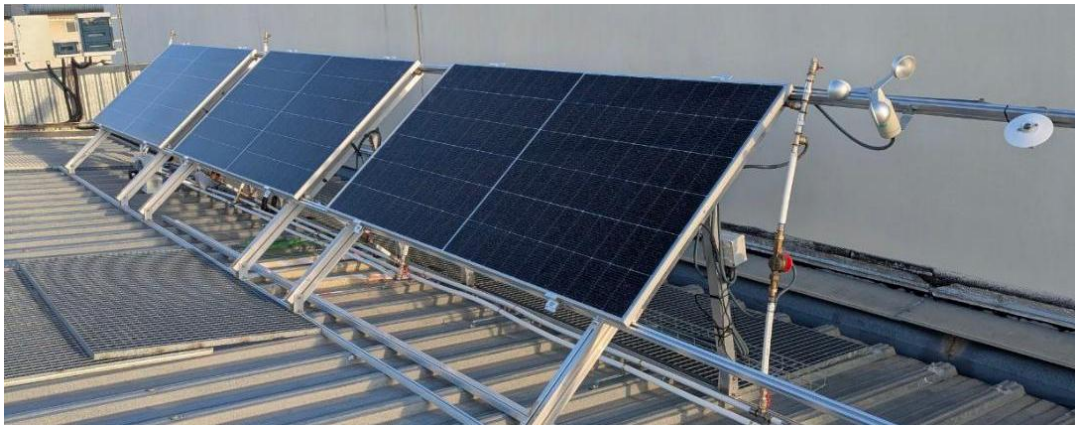
Fig. 1: Frontal side of the test bench, with the three prototypes installed.
