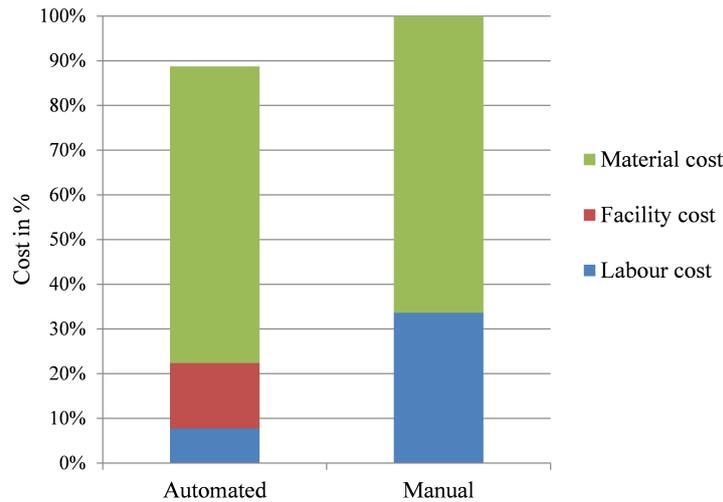
**Figure 7.** Cost comparison of automated and manual FML lay-up
