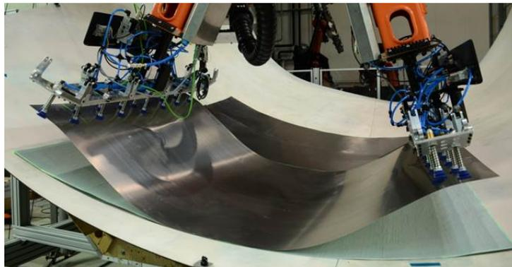
**Figure 2.** Lay-up of two-dimensional aluminium foils with collaborating robots
