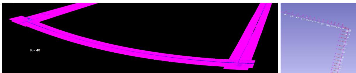
**Figure 5.** Point cloud with detected contour points in blue (left). Visualisation of the target/actual deviation
