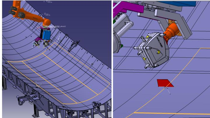
**Figure 4.** CAD model of the mould and the contours of an aluminium layer. The laser light-section sensor is mounted to a robot (left). The laser light-section sensor is moved along the contour (right)
