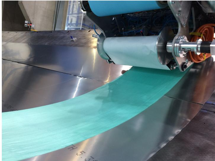
**Figure 3.** Application of glass prepreg
