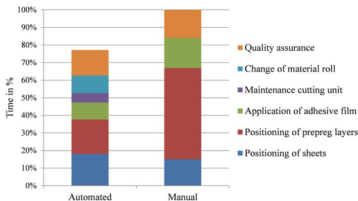
**Figure 6.** Process time comparison of automated and manual lay-up process
