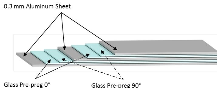
**Figure 1.** Schematic of a 3/2 FML lay-up
