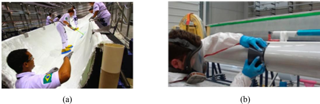
**Figure 2.** (a) Surface textile material application over the in-mould coating before the resin infusion process of a large turbine blade. Depending on the curing conditions of the coated area, its chemical and adhesion relation with the later infused resin is different. (b) Leading Edge Protection application with trowel.
