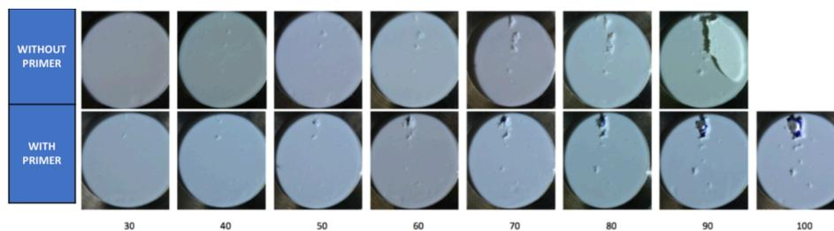
**Figure 9.** Images of surface and delamination damage after time intervals (in minutes) of testing. (upper) LEP coating with No-primer application. (lower) LEP with intermediate primer layer. These results correlate well with the similar erosion incubation time observed in both configurations (with and without primer) in the rain erosion testing. The primer layer avoids delamination but no affect erosion incubation time
