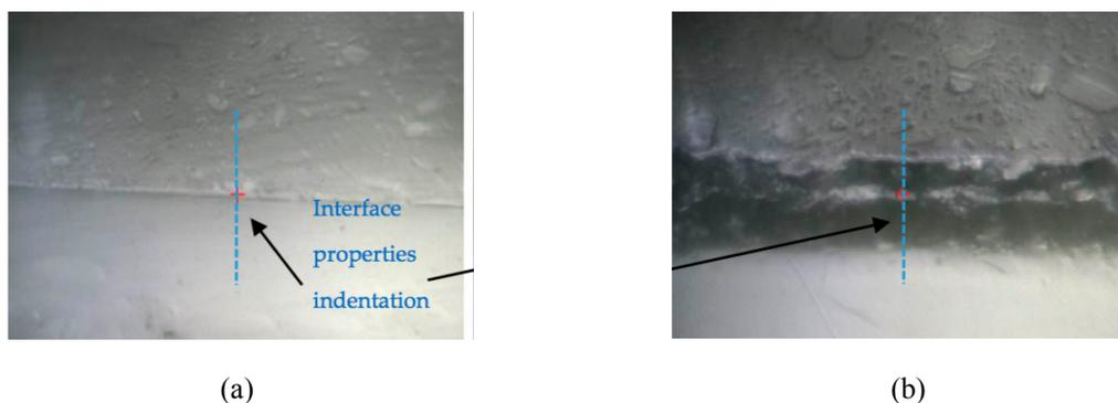
**Figure 3.** Layout of the indentation for Gel Coat and interphase properties of the two cases of curing. (a) Coat 1, i.e. Cured and (b) Coat 2, i.e. Semi-cured.
