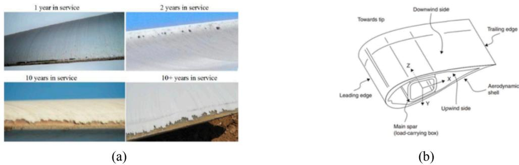
**Figure 1** (a) Examples of leading edge erosion across a range of years in service; (b) blade section with leading edge location where the rain erosion protection is critical.
