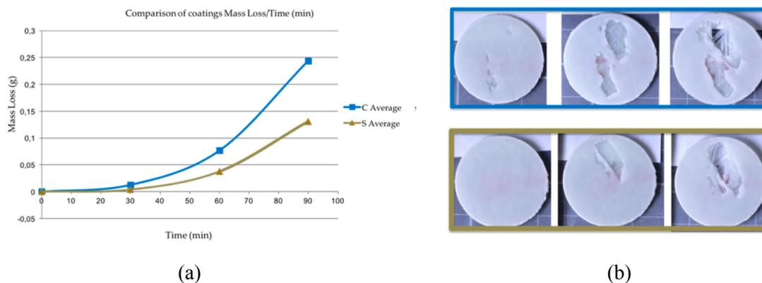
**FIGURE 5.** (a) Average mass loss versus time for two different coatings: Coat 1 i.e. Cured (C in blue) and (b) Coat 2 Semi-cured, (S in Green). (b) Images of surface and delamination damage at 30, 60 and 90 min.
