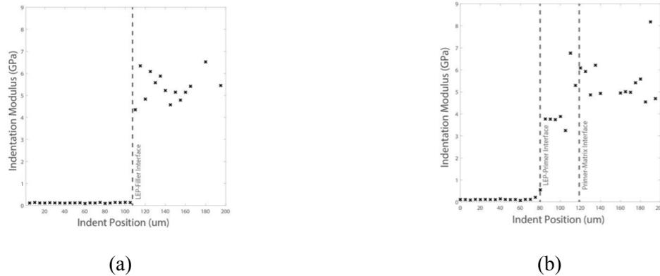
**Figure 8.** Two series of indents reveals (a) a similar acoustic impedance on Primer-Filler interface and (b) shows also how the primer matches the filler acoustic impedance without pronounced discontinuities
