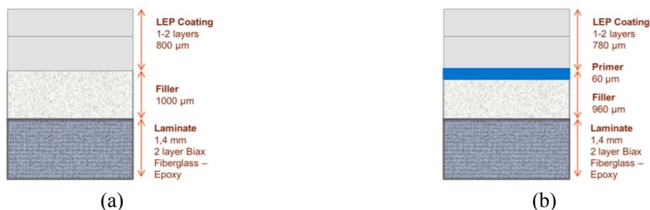
**Figure 7.** (a) Leading Edge Protection Coating configuration with an intermediate filler layer. (b) Additional primer layer included to improve adhesion to substrate.
