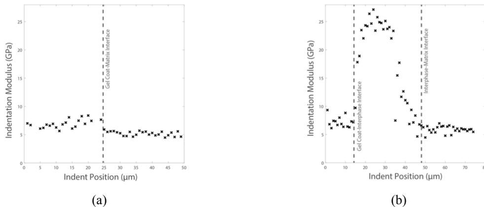
**Figure 4.** Two series of indents across the interface for the two samples of in-mould Gel Coat and the epoxy based matrix of the GFRP laminate with different curing conditions (a) Coat 1, i.e. Cured and (b) Coat 2, i.e. Semi-cured. A clear interphase is present between the materials, where the interphase has a much larger stiffness than either material.
