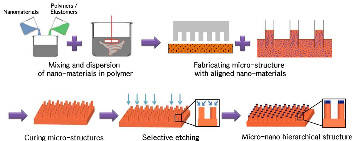
**Figure 1.** New fabricating method of micro-nano hierarchical structures for synthetic dry adhesives
