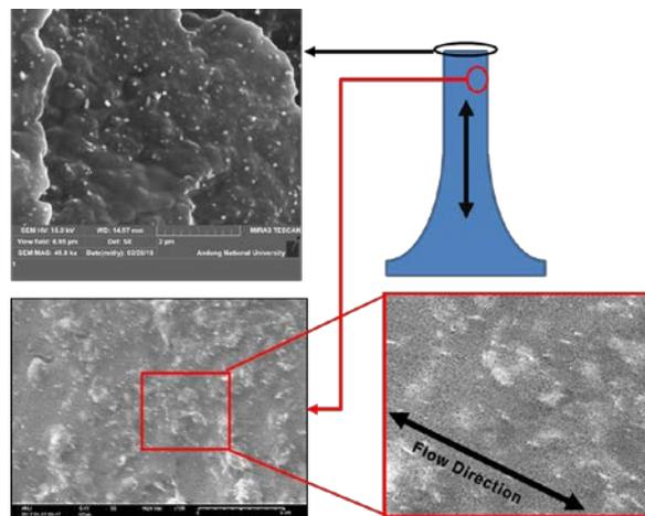
Figure 3. Alignment of MWCTNs within the microstructures
