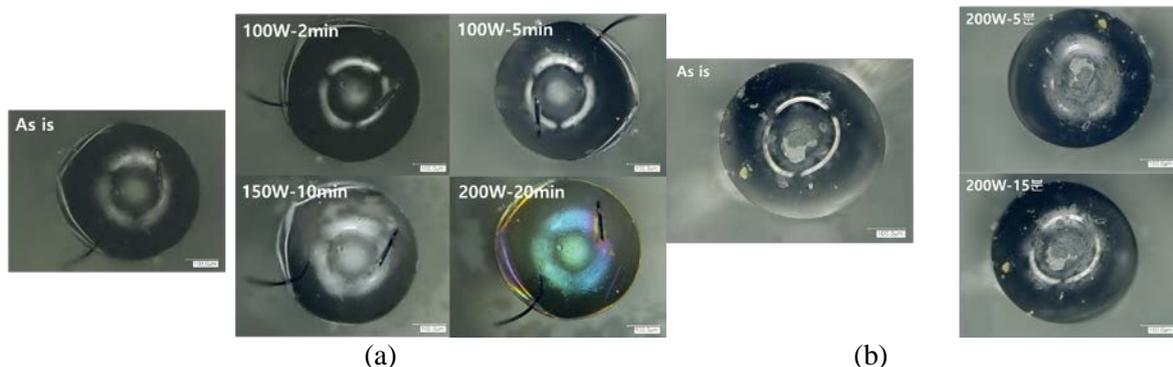
Figure 4. Surfaces of dry-etched microstructures with (a) Nitrogen gas and (b) Oxygen gas.
