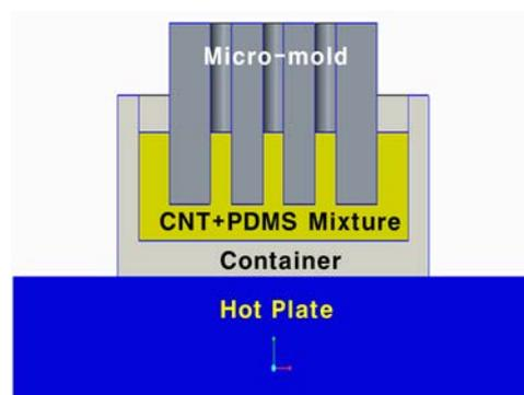
**Figure 2.** Fabricating microstructures of PDMS reinforced by MWCNTs
