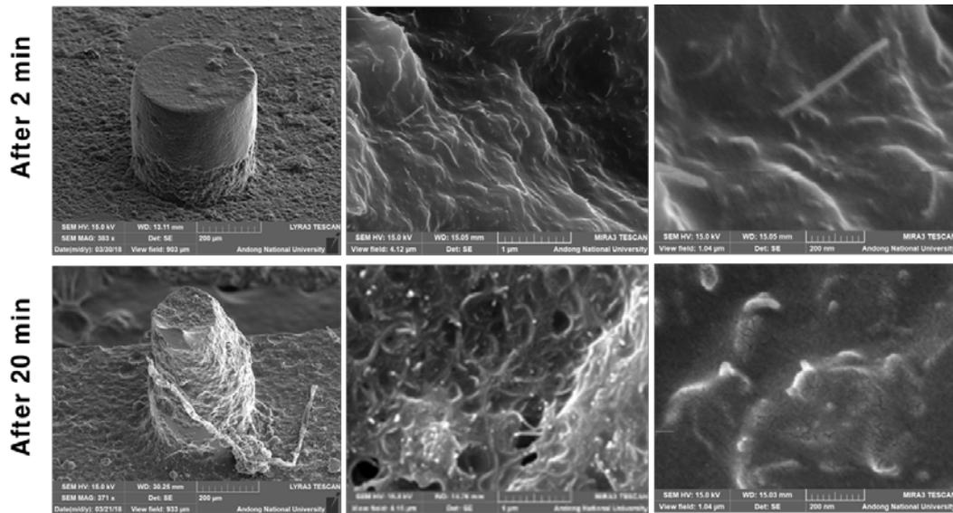
**Figure 5.** Surfaces of wet-etched microstructures reinforced by 1wt% of MWCNTs with respect to the treatment duration.
