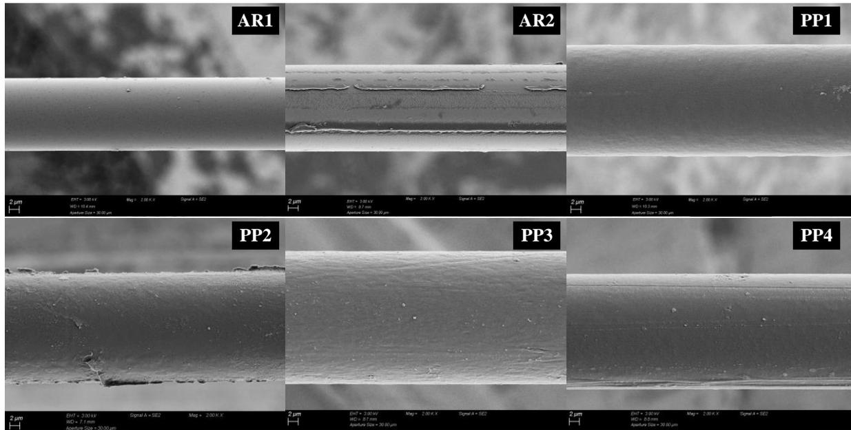
**Figure 1.** SEM images of the surface of all investigated fibres before the pull-out test: AR1 and PP1 without sizing, AR2/PP2-PP4 sized
