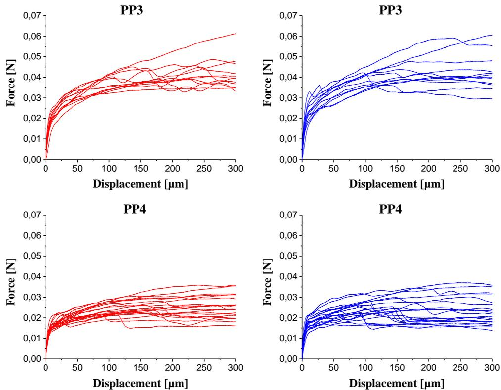
**Figure 4.** Force-displacement curves of the dynamic pull-out tests: PP3 and PP4 fibres embedded in C2 (red), PP3 and PP4 fibres embedded in C3 (blue)
