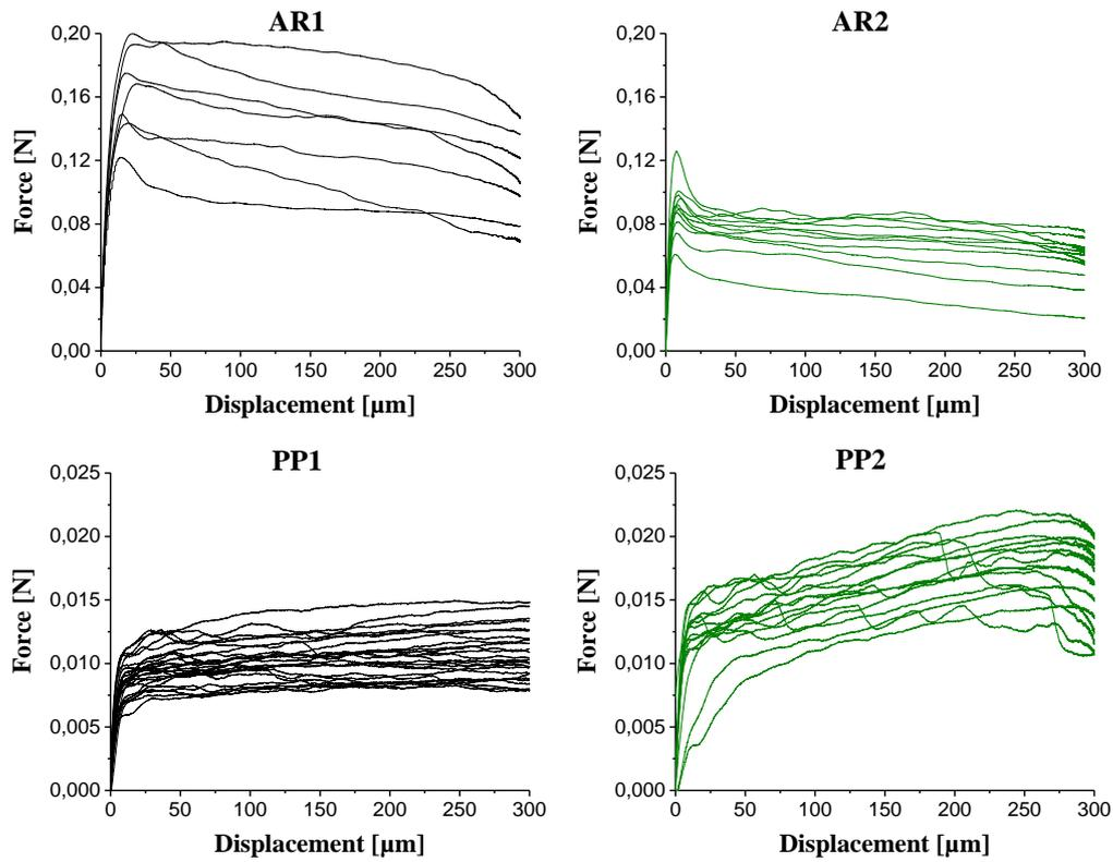
**Figure 3.** Force-displacement curves obtained by the dynamic pull-out tests: AR1 and PP1 fibres without sizing embedded in C1 (black), AR2 and PP2 fibres with PP sizing embedded in C1 (green)
