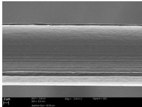
**Figure 6.** SEM image showing the plastic deformations on the surface of PP3 fibre (in comparison to the initial fibre, see Figure 1) embedded in C2 matrix after quasi-static pull-out test
