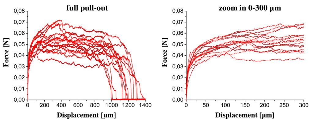
**Figure 5.** Force-displacement curves obtained in the quasi-static pull-out tests on PP3 fibre embedded in C2 matrix
