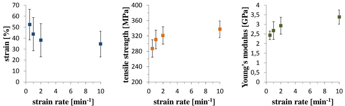
**Figure 2.** Strain, tensile strength and Young's modulus of PP3 fibre in dependence of the strain rate
