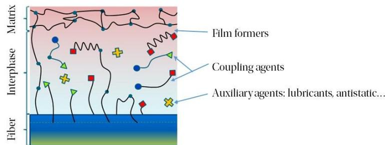
**Figure 1.** Schematic representation of the interphase due to sizing treatment of the fiber.
