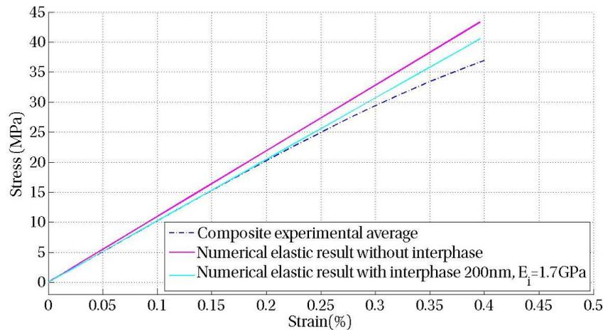
**Figure 8.** Experimental and numerical comparison.
