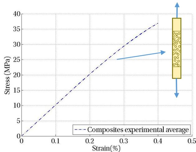
**Figure 2.** Composite mechanical behavior, transverse traction.
