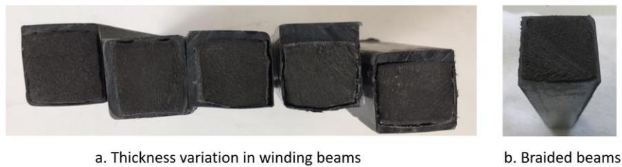
**Figure 9.** Thickness variation in wound beams and braided beam
