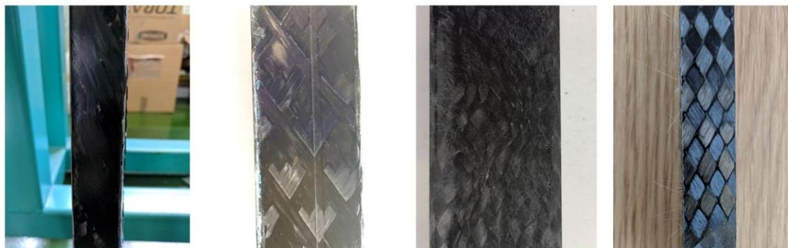
a. Fibre distortion in winding beam    b. Winding beam    c. Fibre distortion Braided beam    d. Braided beam
