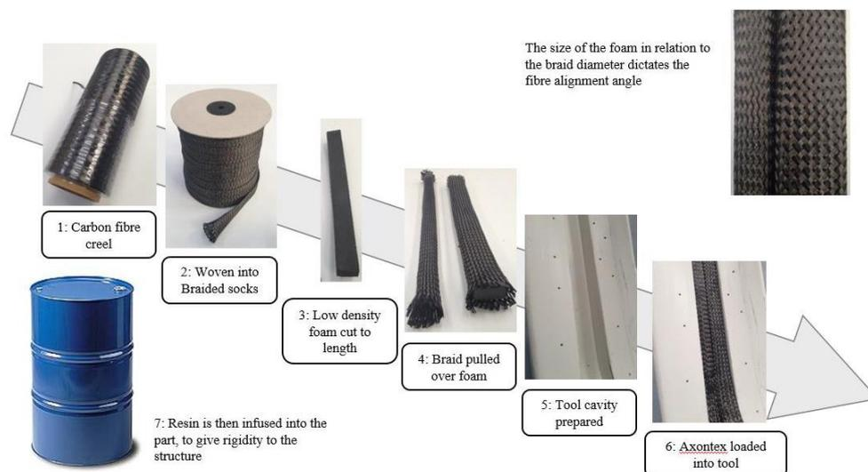
**Figure 6.** Braiding and beam manufacturing process of Axontex™ beam [5].
