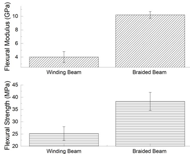
**Figure 11.** Flexural strength and flexural modulus of wound and braided beams
