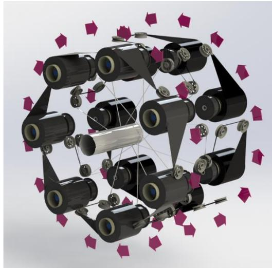
**Figure 2.** Ring winding mechanism
