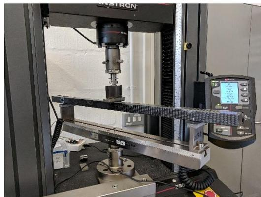
**Figure 10.** Three point bending test setup
