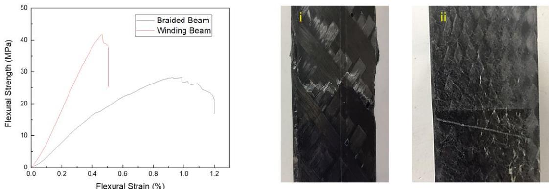
a. Flexural strength– flexural strain curve    b. Crack development (i--winding beam, ii—braided beam)
