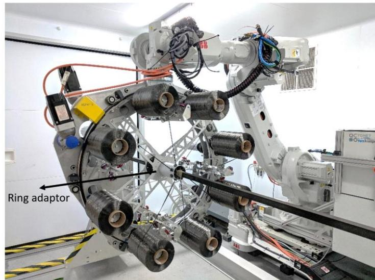
**Figure 5.** Winding process of Axontex™ beam using 3D complex winding machine in Cygnet Texkimp
