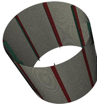
**Figure 1.** Finite element model of stiffened cylinder
