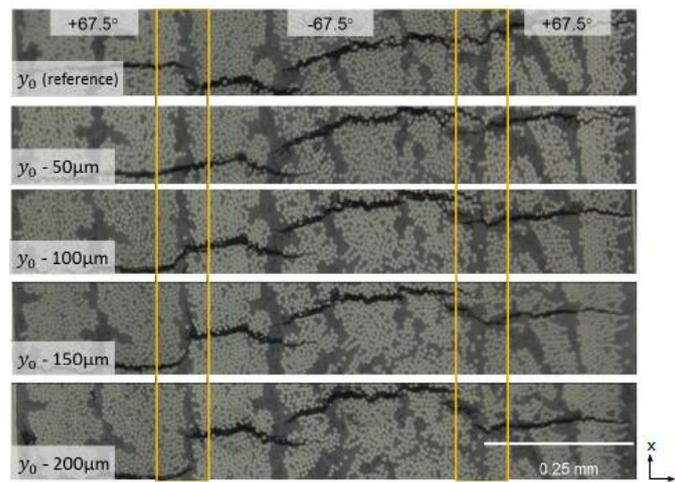
**Figure 6 :** Intersection between the cracks of three plies in a  $[0/+67.5/-67.5]_s$  for five polishing depth, the yellow boxes highlight the two interfaces
