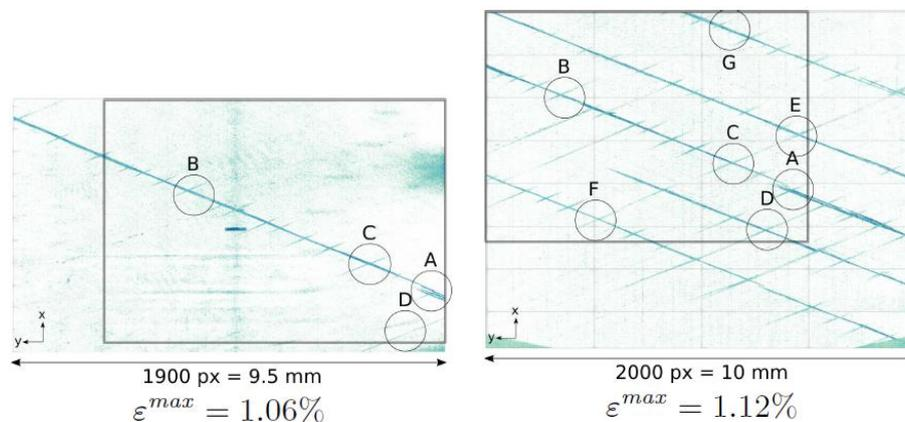
**Figure 4.** Illustration of the evaluation of the number of crack crossings between two plies
