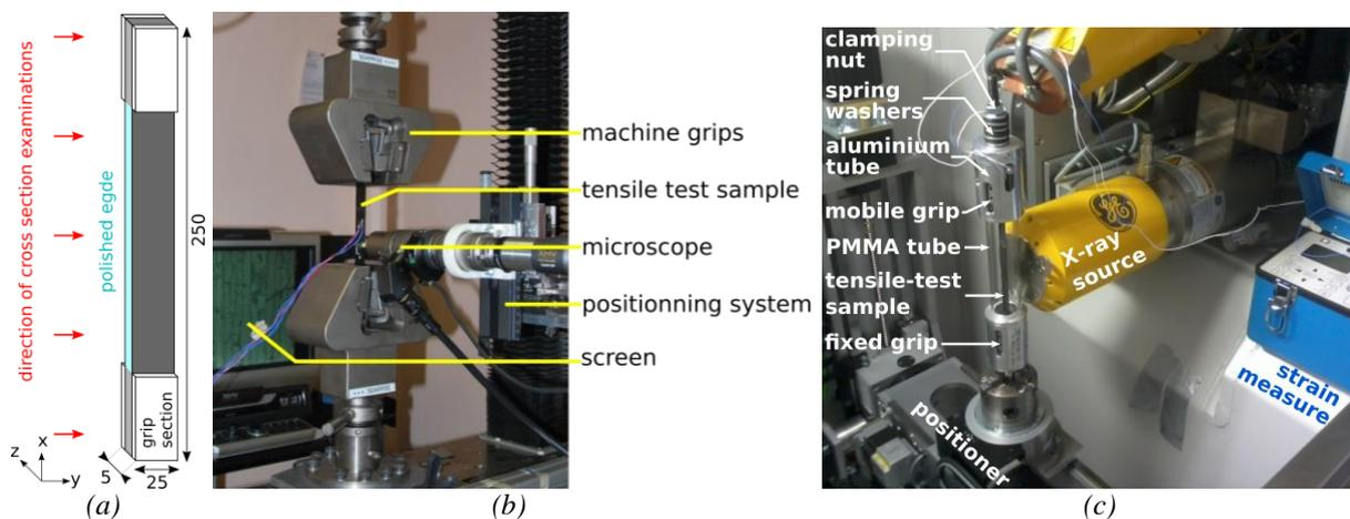
**Figure 2.** (a) Dimensions of specimens, (b) Damage observation under tensile loading test, (c) Observation device under traction loading placed in tomograph
