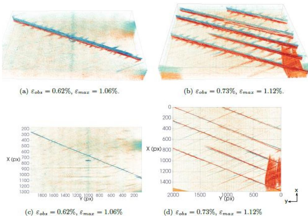
**Figure 3.** 3D reconstruction by thresholding a network of cracks for two maximum strains, two colors are assigned to the cracks to differentiate the two interfaces
