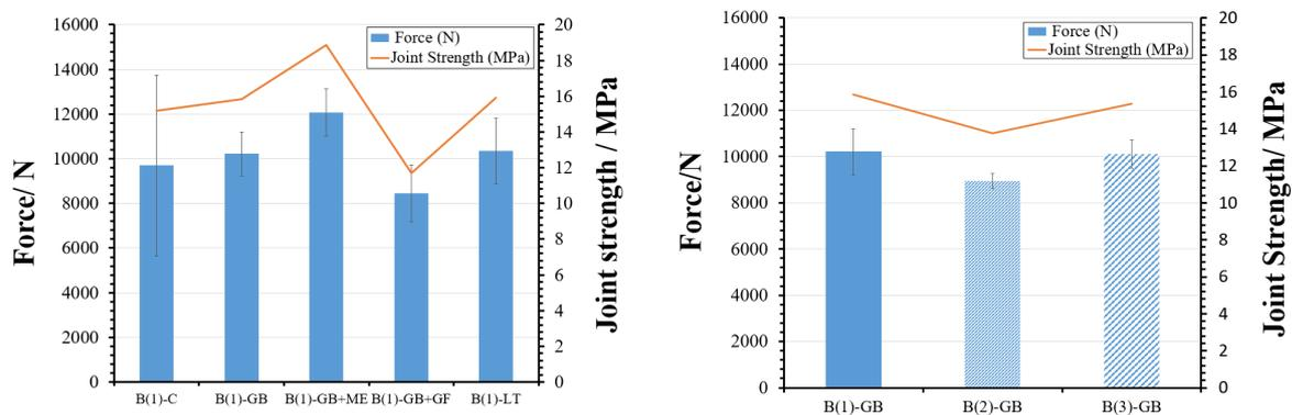
**Figure 4.** shear strength of single lap joints of system B (left) with different surface conditions and (right) different processing cycles.
