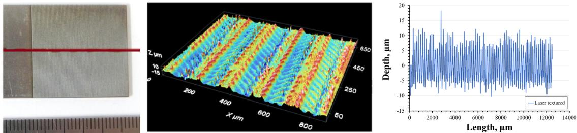
**Figure 2.** (from left to right) picture of a textured surface, 3D confocal maps and 2D profile obtained by means of a contact profiler.
