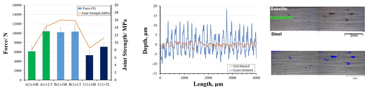
**Figure 3.** (from left to right) shear strength of single lap joints, 2D profile for grit blasted and laser textured surfaces, and cross section of the joints manufactured including porosity quantification.
