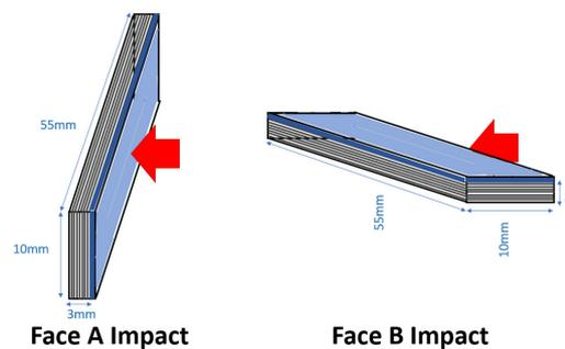
**Figure 1.** Schematic of the impact test performed on the multimaterial components where the orientation of the sample related to the impactor is displayed. The red arrow stands for the the impactor, whereas blue indicates the AHSS steel and the stacking sequence is represented in grey.
