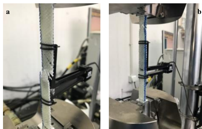
Figure 12. Tensile coupons fixated on the testing machine. (a) prior to failure (b) post-failure
