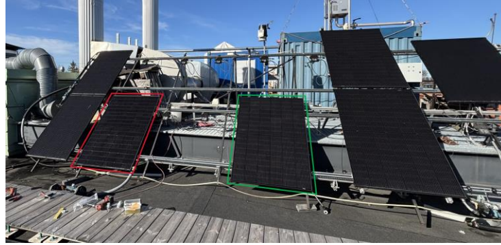
Fig. 2: PVT outdoor testing facility with prototype collector (red) and reference panel (green)
