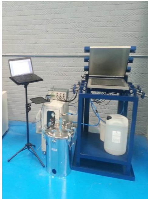
Figure 2. Experimental set-up for measurement of in-plane permeability.
