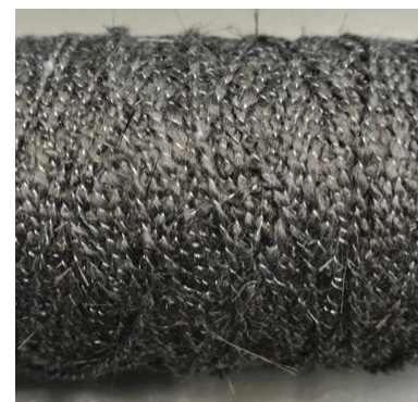
Figure 5. Final hybrid yarn (800tex)
