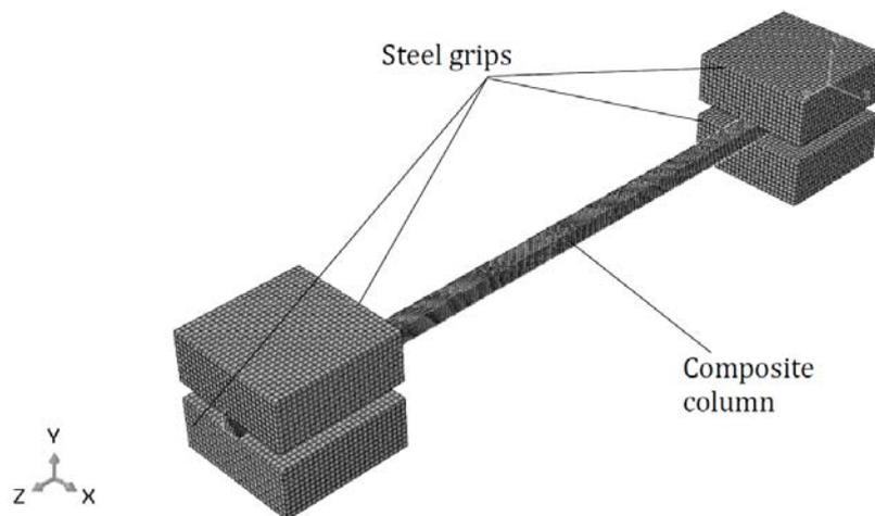
**Figure 1.** 3D view of the finite element model with a gauge length of 200 mm. This model was used to calculate stress concentrations due to the grips.
