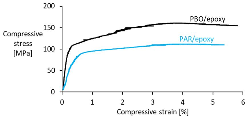
**Figure 2.** Compressive stress-strain diagrams of PBO/epoxy and PAR/epoxy revealing their poor compressive performance.
