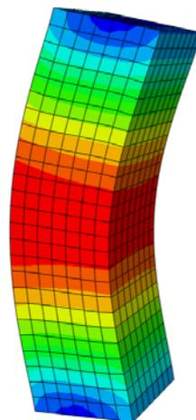
**Figure 3.** Example of the finite element model predicting buckling for gauge lengths below those predicted by the equation in ASTM standard D3410.
